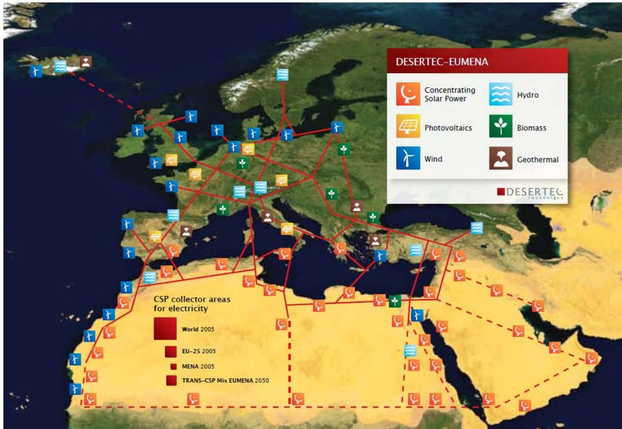
Figure 36. Concept of a “EUMENA Supergrid” based on HVDC power transmission as “Electricity Highways” to complement the conventional AC electricity grid, as developed by TREC in 2003. The symbols for power sources and lines are only sketching typical locations. Reprinted from Deserotec Foundation 2009.
