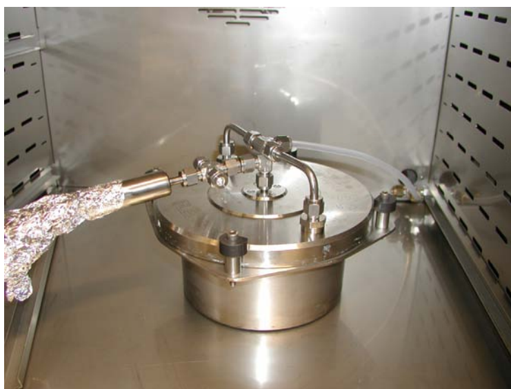
Picture 1. The FLEC chamber.
