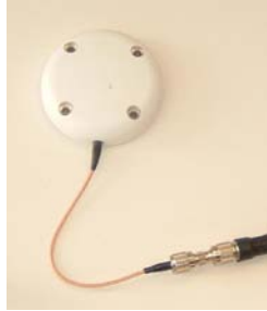
Figure 4. LocaLite (pseudolite) antenna used in indoor positioning trial at UNSW Snap Lab.
