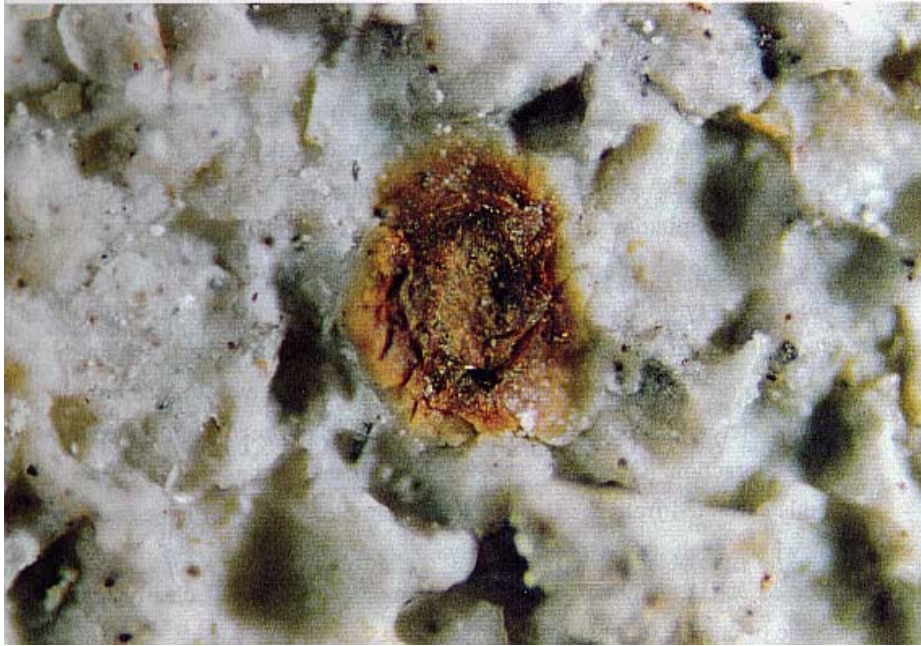
Figure 12. Micrograph of reacted bentonite surface (case A, 36 months) showing the concentric precipitation of ferric compounds around pyrite. Magnification 40 x (after Melamed & Pitkänen 1994).
