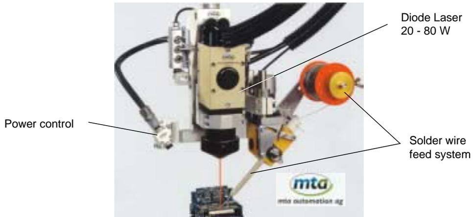
*Figure 10. Scheme of a laser soldering system [35].*
