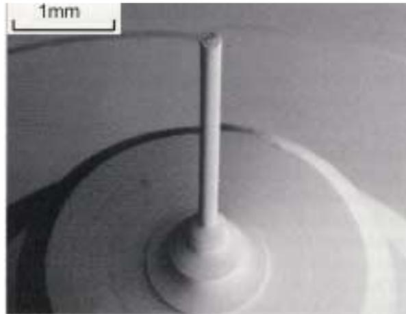
*Figure 1. Photograph of a microcylindrical part, a turned work piece. Hardened die steel, HRC44,  $\text{Ø}0.22 \times 4$  (Moriwaki and Shamato, 2000).*
