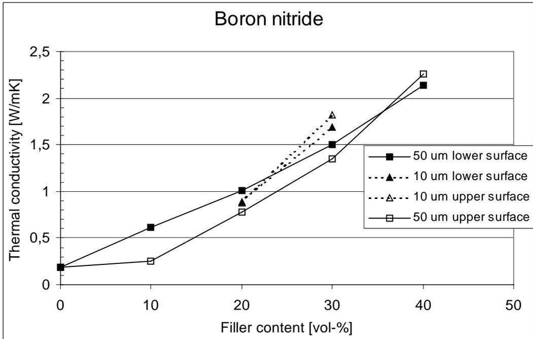
Figure 3. The effect of boron nitride particle size and concentration on the thermal conductivity of boron nitride filled gel.
