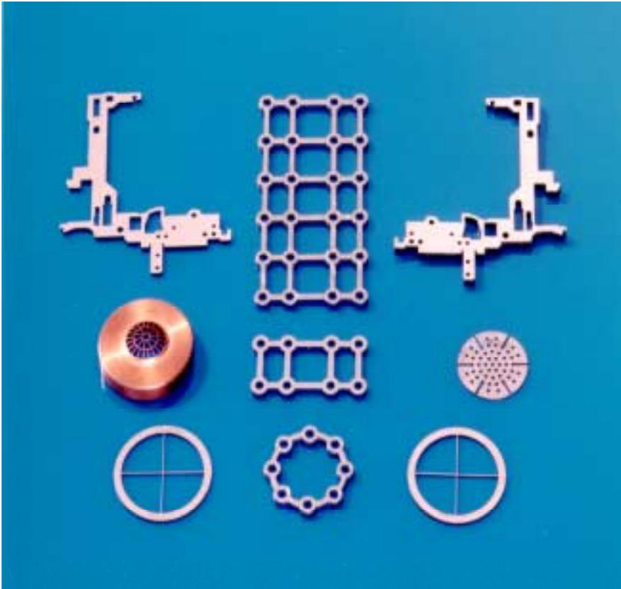
*Figure 1. A variety of metals can be cut with high precision. Material thickness is 0.2–1.5 mm [1].*
