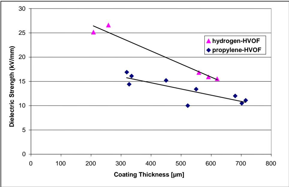
Figure 5. Dielectric strength as a function of coating thickness.
