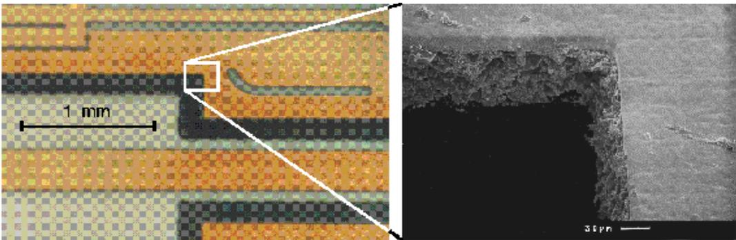
*Figure 3. Precision cuts in a soft substrate using excimer laser radiation [13].*
