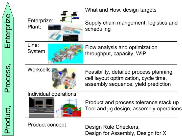
Figure 2. Virtual prototyping and digital plant technologies for design.
