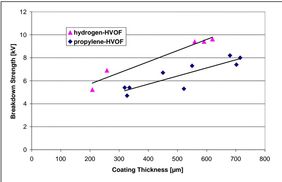
Figure 6. Breakdown voltage as a function of coating thickness.
