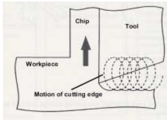
*Figure 3. Schematic illustration of elliptical vibration cutting process (Moriwaki and Shamato, 2000).*
