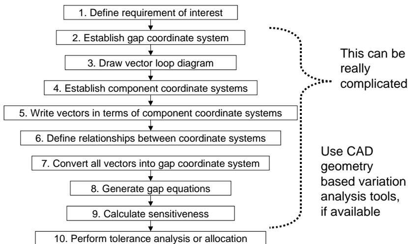
Figure 4. Multidimensional tolerancing flow chart [16].
