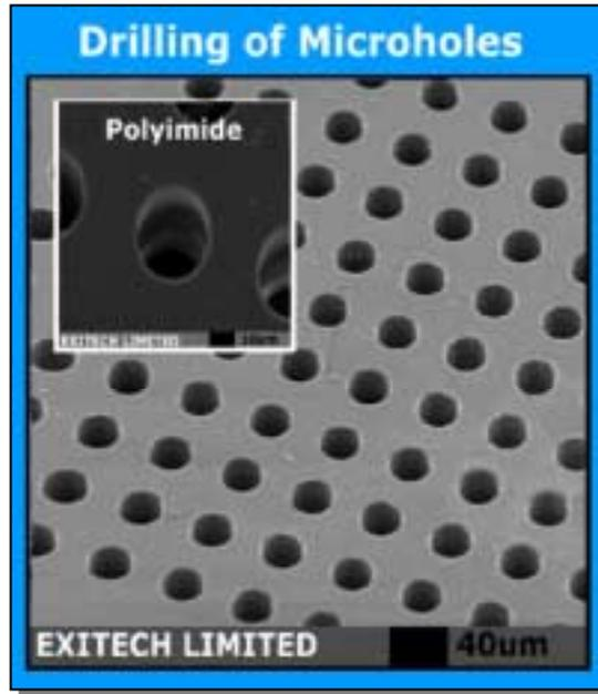
Figure 4. Microholes in polyimide drilled by an excimer laser [11, 16]. Polyimide is used in PCB's and ink jet printers.
