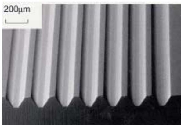
*Figure 2. Photograph of a microgrooved, machined work piece. Hardened die steel, HRC 55 (Moriwaki and Shamato, 2000).*
