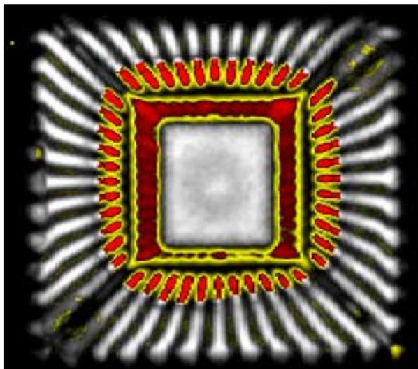
*Figure 5. Acoustic image of a device. The red areas are delaminated.*
