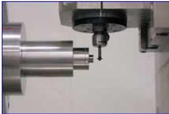
*Figure 5. High-speed spindle for grinding applications (Precitech, 2002).*
