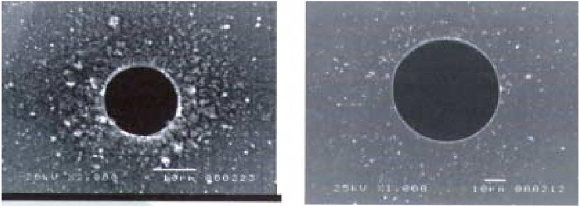
*Figure 5. 17  $\mu\text{m}$  hole 80  $\mu\text{m}$  stainless steel (left) and 40  $\mu\text{m}$  hole in 100  $\mu\text{m}$  stainless steel (right) [20].*
