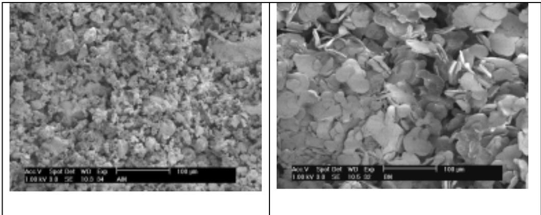
*Figure 1. Scanning electron micrographs of aluminium nitride (left) and boron nitride powder.*
