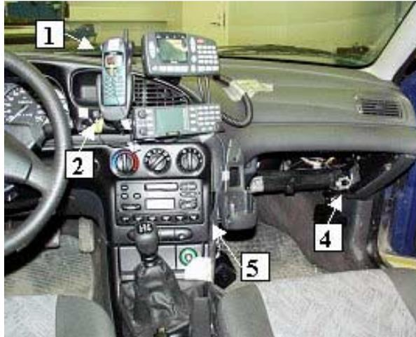
*Figure 3. Determination of shock and vibration environmental conditions in a passenger car. Some of the acceleration measurement locations used are presented (Juntunen et al. 2001).*
