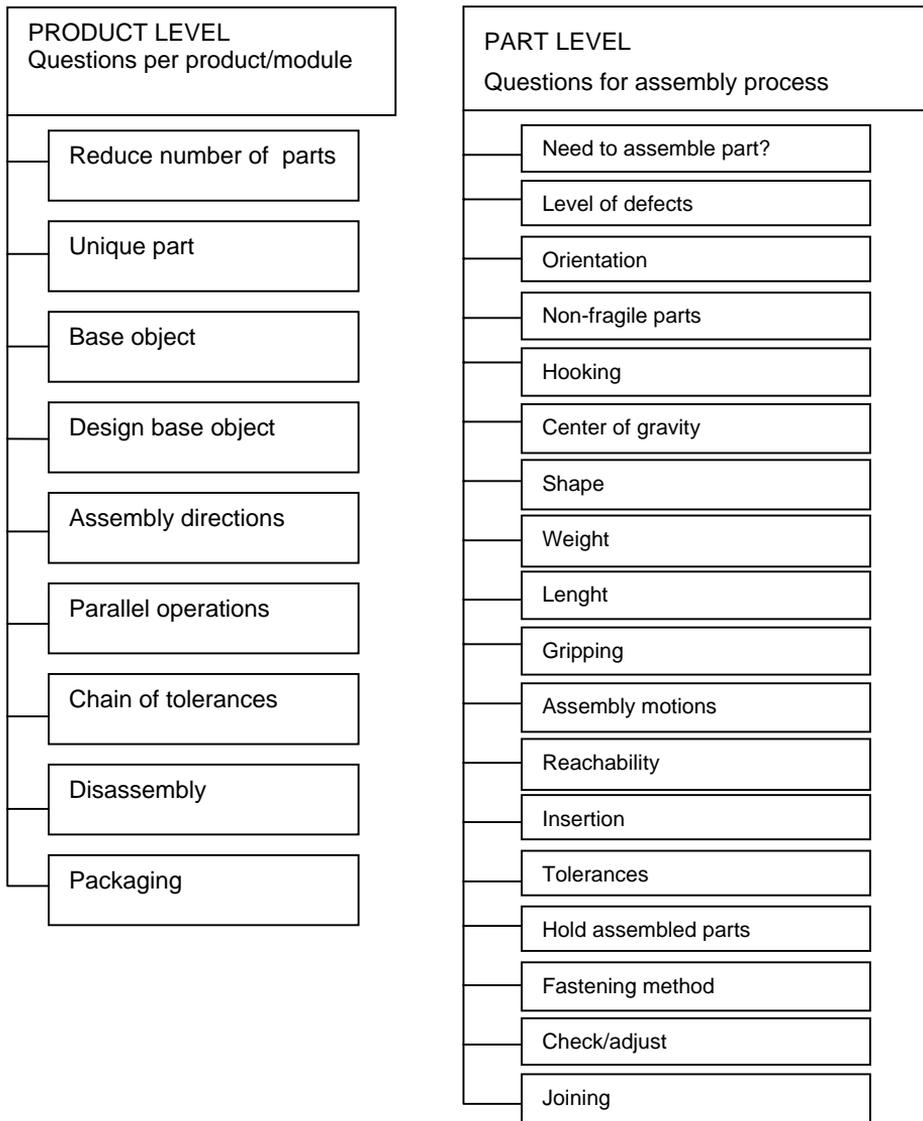
*Figure 3. Design for Automated Assembly Overview [13].*
