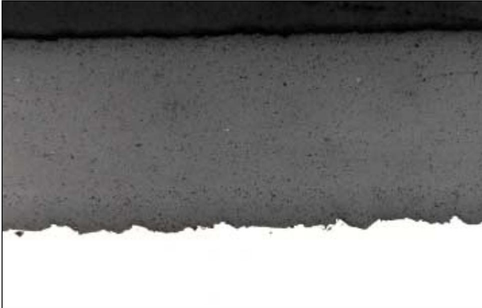
*Figure 4. Cross-section of the 620  $\mu\text{m}$  thick HVOF-sprayed  $\text{Al}_2\text{O}_3$  coating, 100x magnification.*
