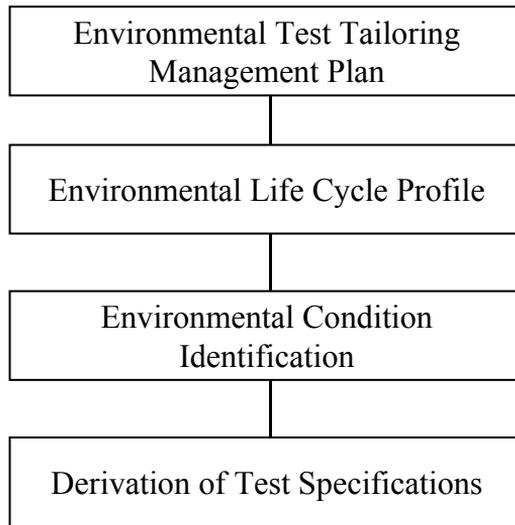
*Figure 1. The main test tailoring process.*
