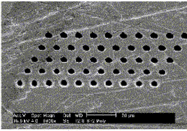
*Figure 7. 5 μm holes in molybdenum sample [26].*
