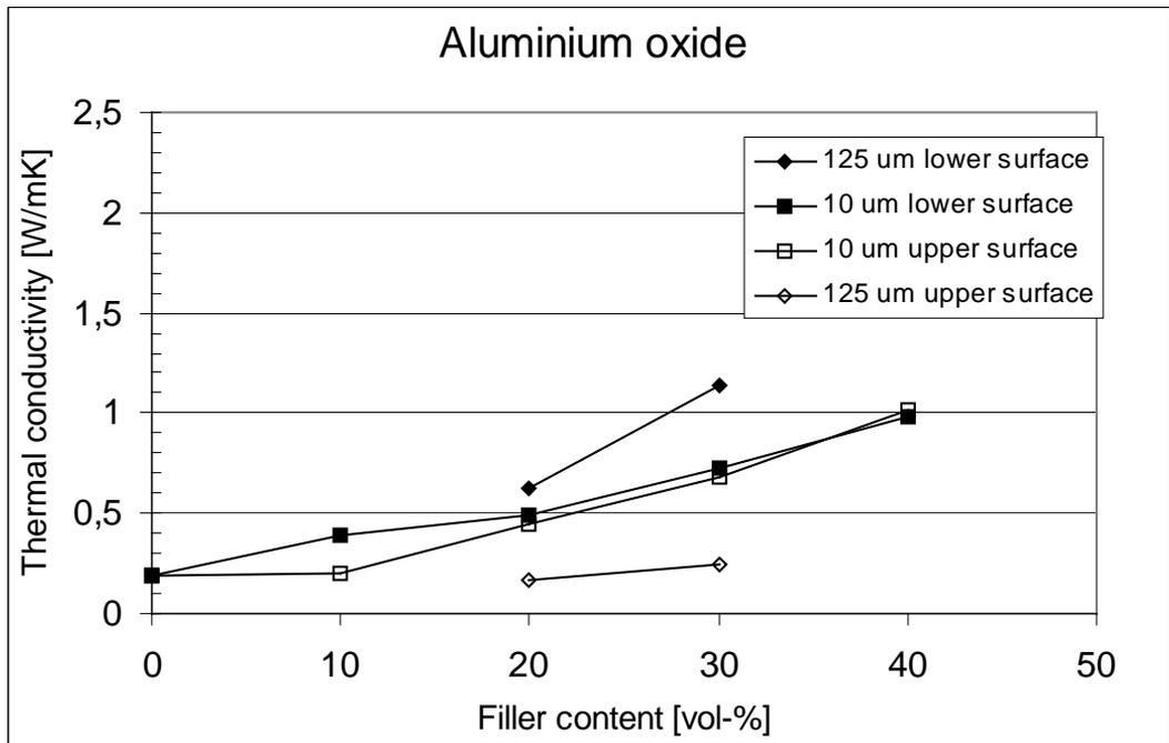
Figure 2. The effect of particle size and concentration of aluminium oxide on the thermal conductivity of gel composite material.
