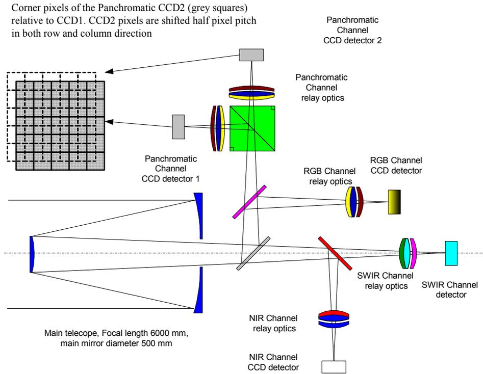
Figure 4. Kioto+ Payload concept based on 500 km altitude and 0.5 m ground resolution achieved with staggered 2 dimensional CCD detectors.
