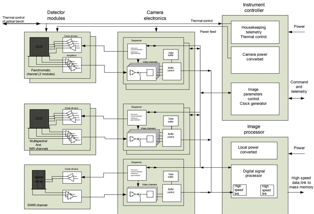
Figure 6. Block diagram of electrical system of the Kioto+ payload.
