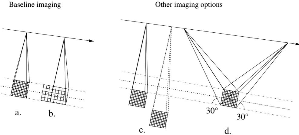
Figure 3. Baseline and optional imaging modes: a. Baseline sample imaging at 0.5 m (panchromatic), 2 m (visible and NIR) and 4 m (SWIR) resolution. b. Continuous-strip baseline imaging over the oceans (100 metre resolution for all channels). c. Possible off-nadir. d. stereoscopic imaging modes. All imaging modes are available for both baseline and optional two-satellite configuration.
