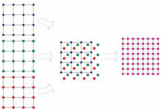
Figure 5. The principles of the super-resolution image reconstruction. First, a sequence of images is taken from the same target with the mutual sub-pixel shifts. Then a thicker super-resolution grid is created and pixel values are interpolated from the single images.
