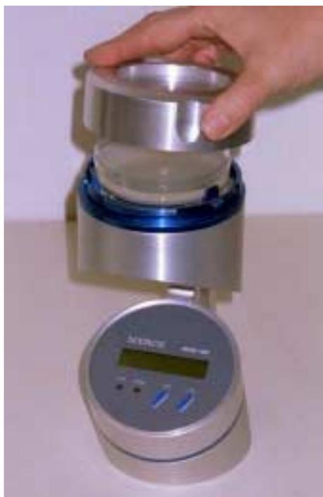
*Figure 7. The MAS-100 air sampler is an impactor.*
