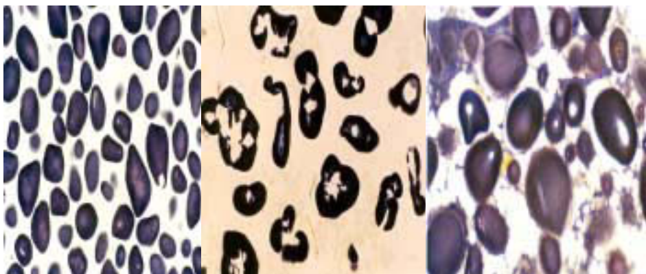
Fig. 12. Native raw potato starch granules (left), hydrolysed granules (middle) and amylose-coated hydrolysed granules (microscopy cross-sections, iodine colour, thickness 4 \mu\text{m} , 290 \times ).
