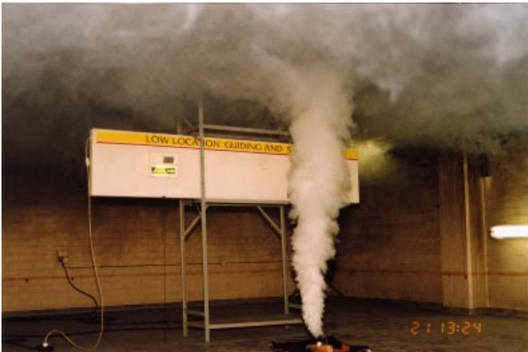
Figure 6. Smoke generation with a smoke bomb.
