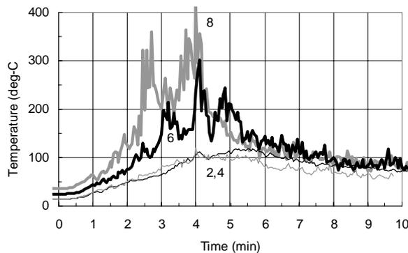
c) Temperatures at the doorway between the fire room and the entrance room at the bottom level (T14).
