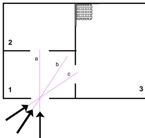
*Figure 15. The three different directions of the fan.*
