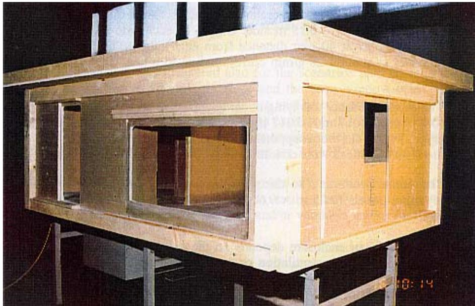
*Figure 2. The first version of the test compartment from outside. In final tests the fire room walls were made of Siporex (see Figure 4), and there was no observation window in front because the tempered glass broke during the preliminary tests.*
