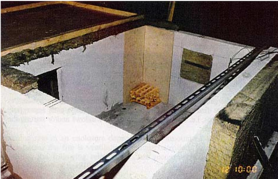
*Figure 4. The fuel package in the corner. The fire room walls are made of Siporex tiles, and the two windows are closed with pieces of glass wool.*
