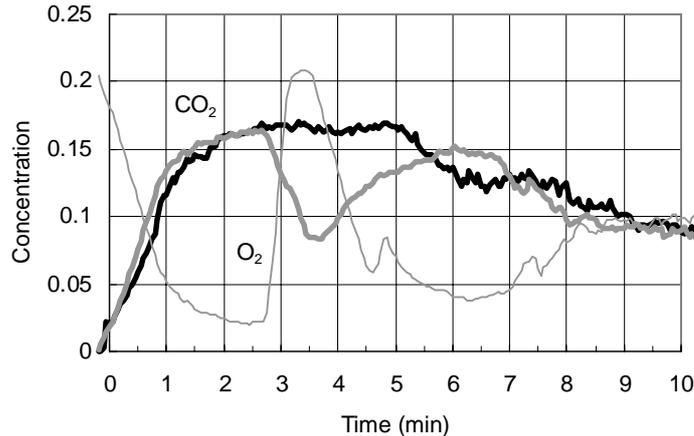
*If the window is open in the fire room, opening the door does not mix the gases in any significant way, whereas in the case of having the target room window open, opening the door abruptly provides more oxygen to the “starving” fire and initiates strong gas flows and mixing in the fire room.*
