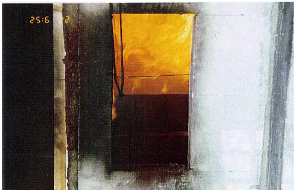
*b) With PPV the gas layers and flames are mixed in the fire room. The flames are pushed away from the entrance door opening. (ST34)*
