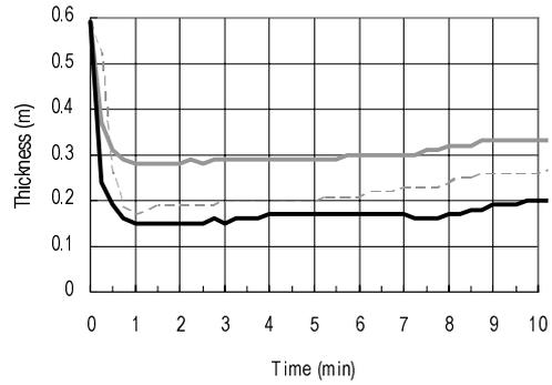
d) Lower layer thickness in the compartment.
