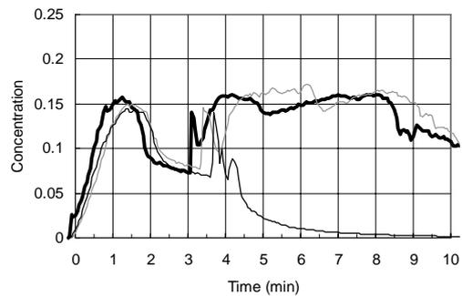
c) CO<sub>2</sub> concentration close to the ceiling level in the fire room.
