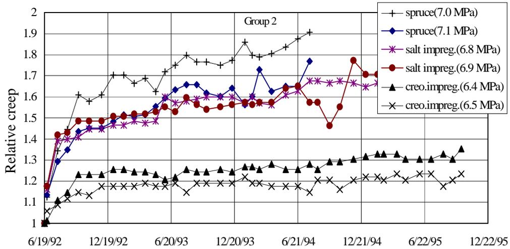
Figure 11. Relative creep versus time for samples in group 2.
