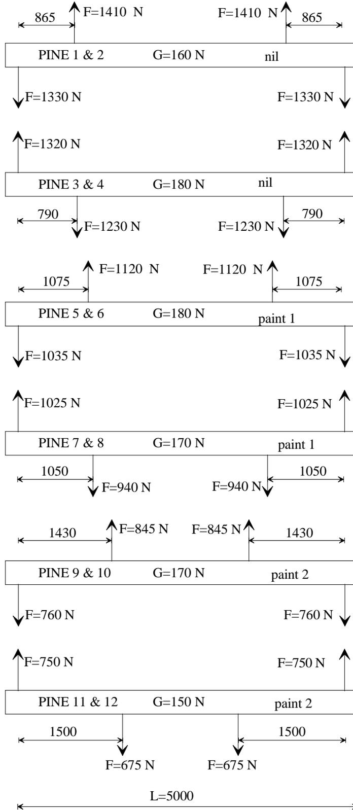
Figure 4. Schematic of loading and supporting system for group-1 specimens.
