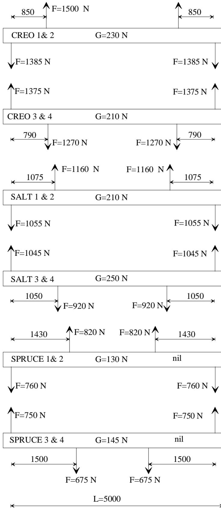
Figure 5. Schematic of loading and supporting system for group-2 specimens.
