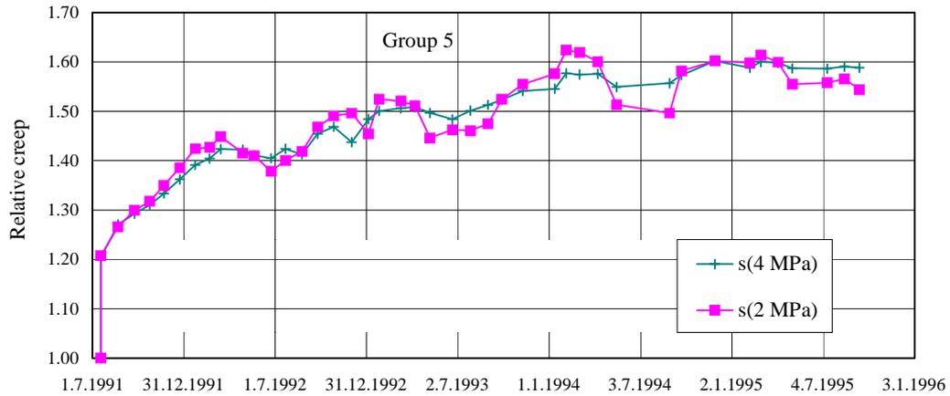
Figure 17. Relative creep (mean of 4) versus time for glulam in heated room for different load levels (2 and 4 MPa).
