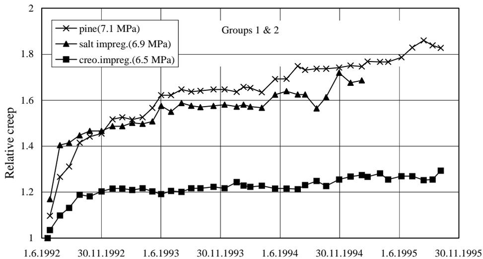
Figure 12. Average relative creep versus time for untreated and impregnated pine.
