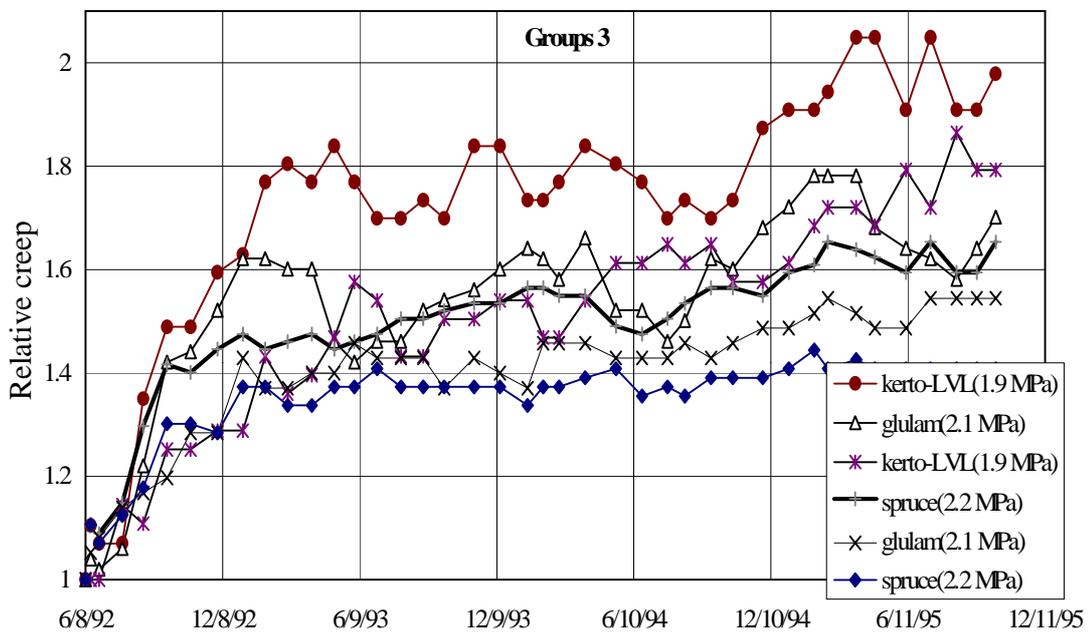
Figure 13. Relative creep versus time for specimens in group 3.
