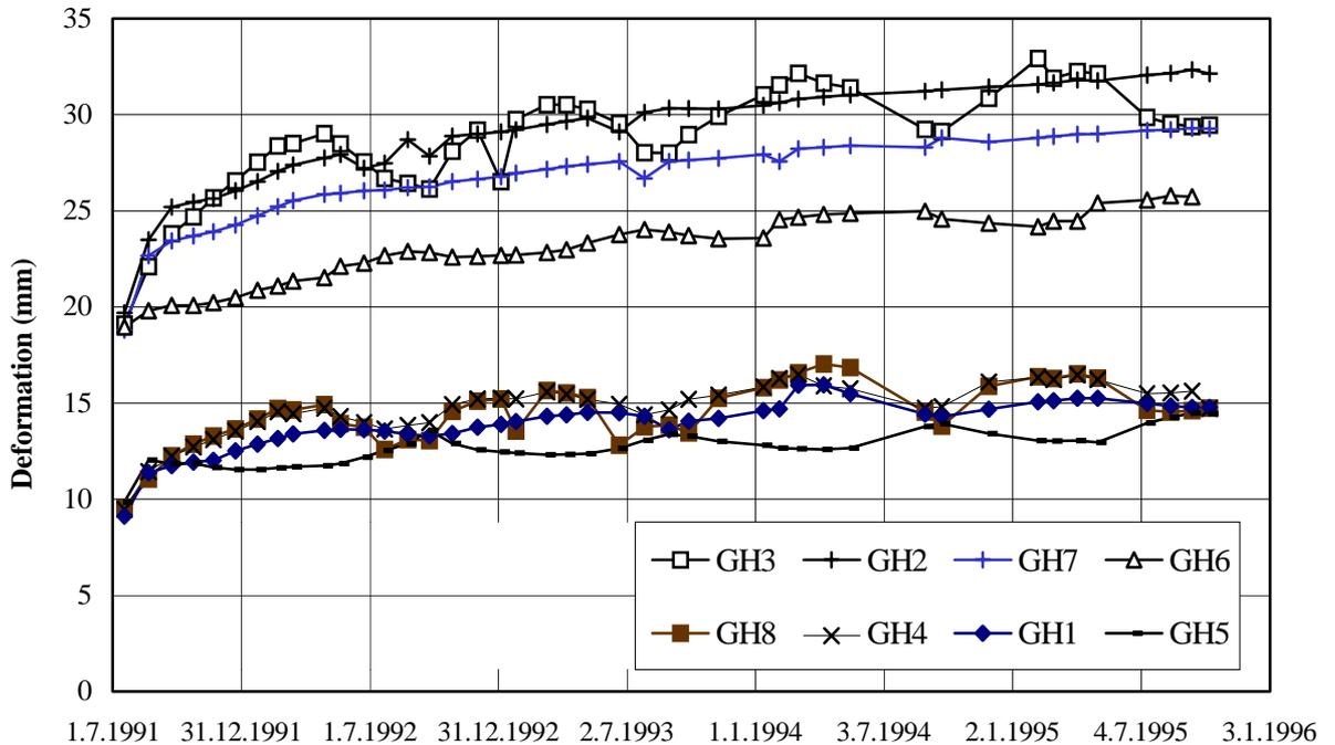
Figure 16. Total deflection versus time for specimens in group 5 (Glulam beams).
