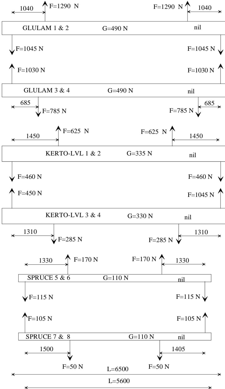
Figure 6. Schematic of loading and supporting system for group-3 specimens.
