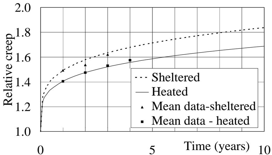
Figure 28. Prediction of creep by eqn.(1) based on observations after one and two years.
