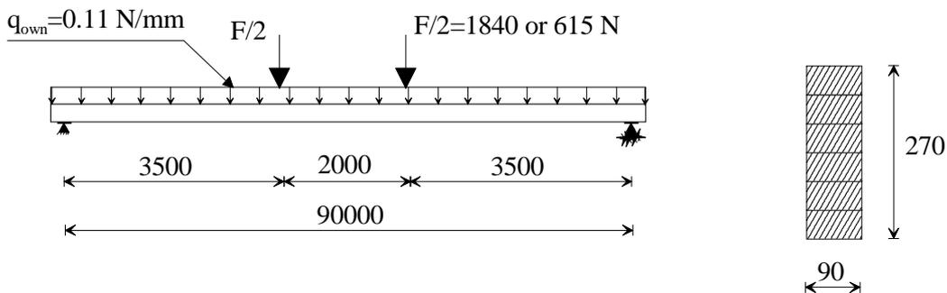
Figure 8. Loading and supporting systems for glulam beams in heated room.
