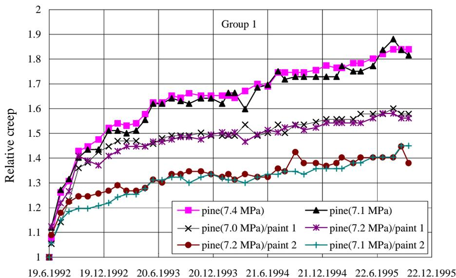
Figure 9. Relative creep versus time for specimens in group 1.
