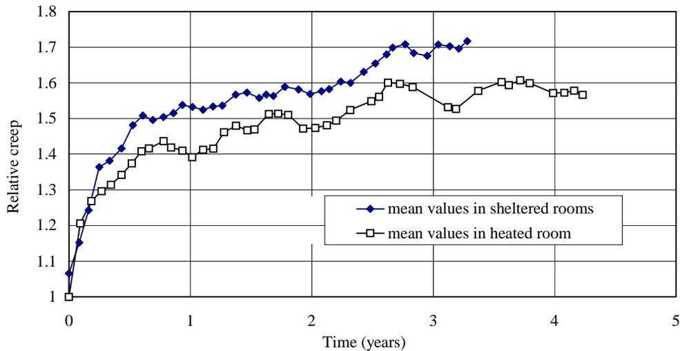
Figure 18. Comparison of average relative creep versus time (glulam specimens in heated room and other samples in sheltered rooms).
