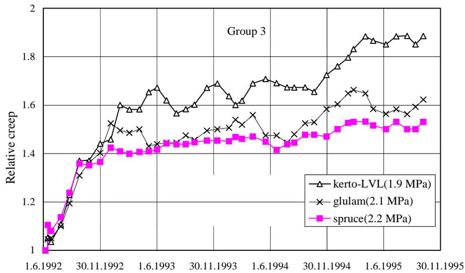
Figure 14. Average relative creep versus time for specimens at lowest load levels.
