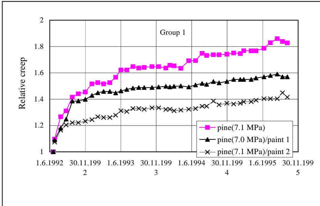
Figure 10 Average relative creep for different surface coatings.
