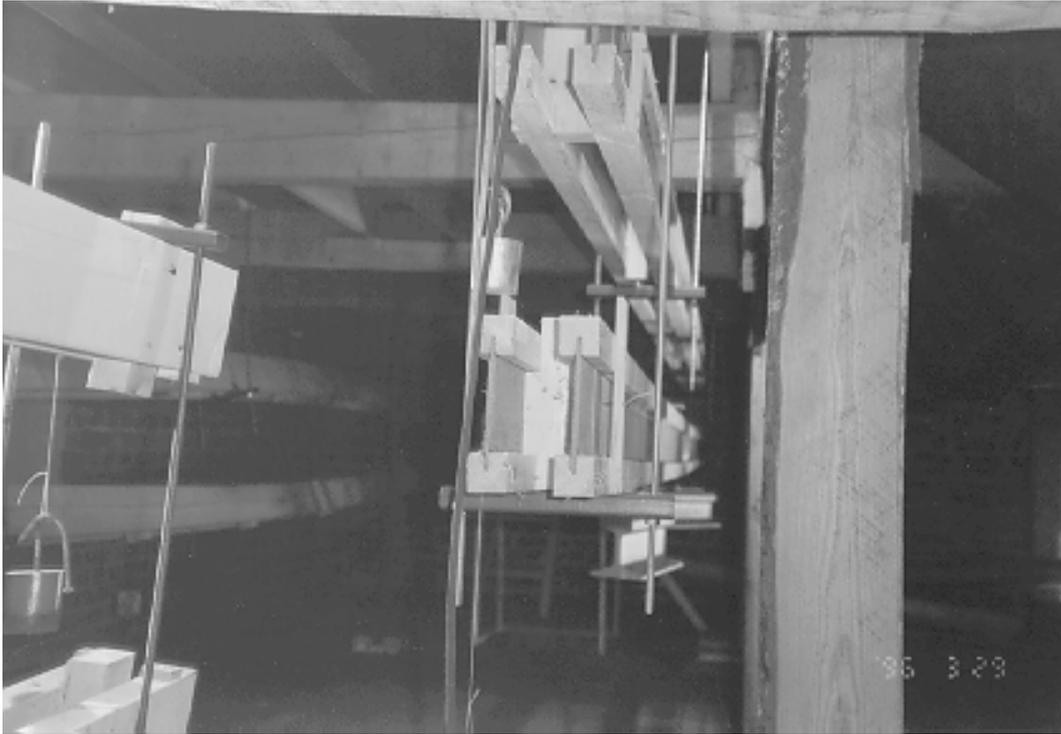
*Figure 3 Photograph of test set-up and loading arrangements in sheltered environment for I-beams in group 4.*
