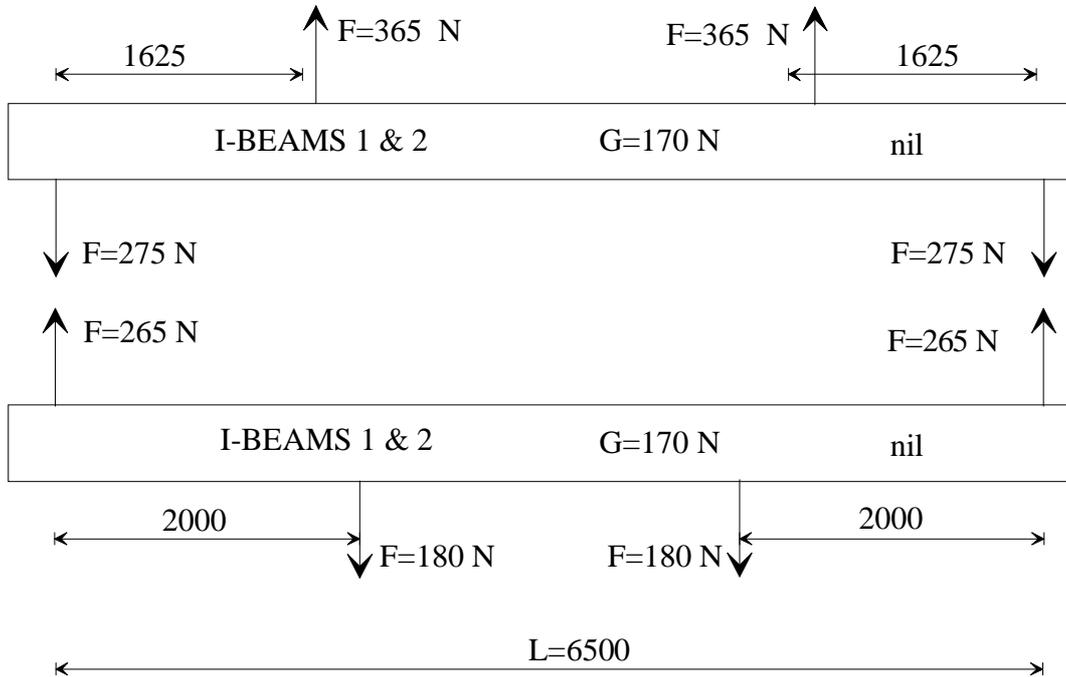
Figure 7. Schematic of loading and supporting system for group-4 specimens.
