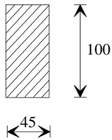
*Figure 1. Schematic of specimen configurations used in non-heated environment.*
