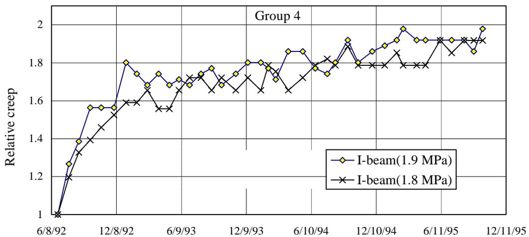
Figure 15. Relative creep versus time for specimens in group 4.
