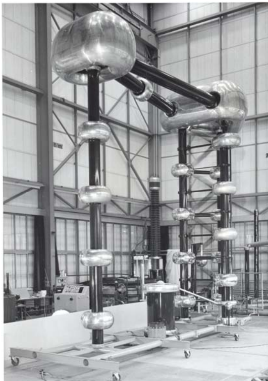
Figure 1. Left: The 1200 kV HVDC system at Aalto University. Generator on the back and the divider on the front. Right: Aalto divider on the right and MIKES 200 kV reference divider on the floor on the left.
