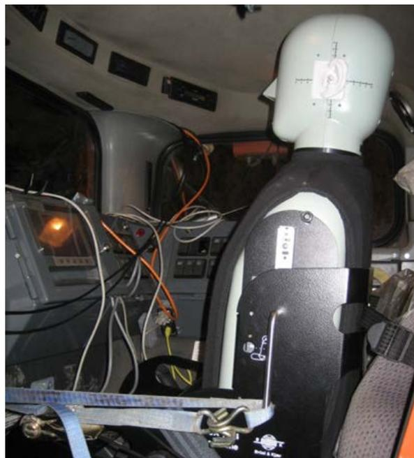
**Figure 3: Binaural recording setup inside the LHD cabin.**
