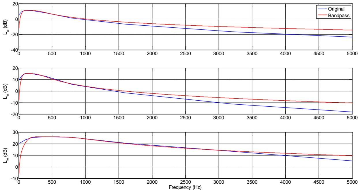
**Figure 8: Ventilation noise spectra for minimum flow speed (up), half speed (center) and maximum flow speed (low).**
