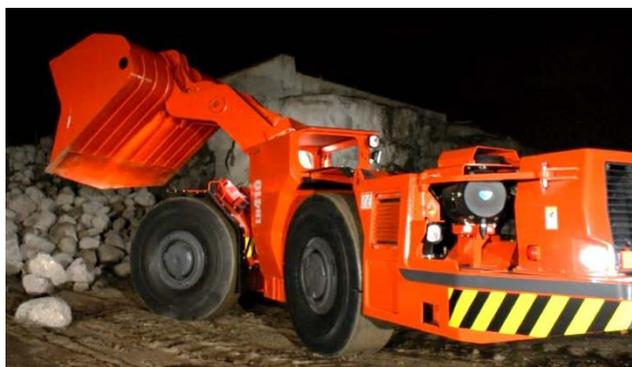
**Figure 1: Sandvik LH410 (formerly Toro 7) Loading and Hauling Device, LHD. Photograph courtesy of Sandvik [8].**
