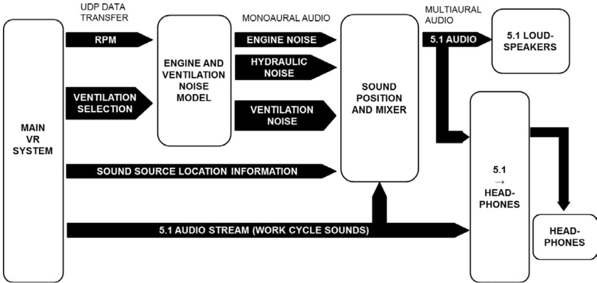
**Figure 6: Audible Model Platform (AMP) for the LHD cabin noise model. The sources of noise are engine orders, hydraulics orders, engine broadband noise and ventilation noise.**
