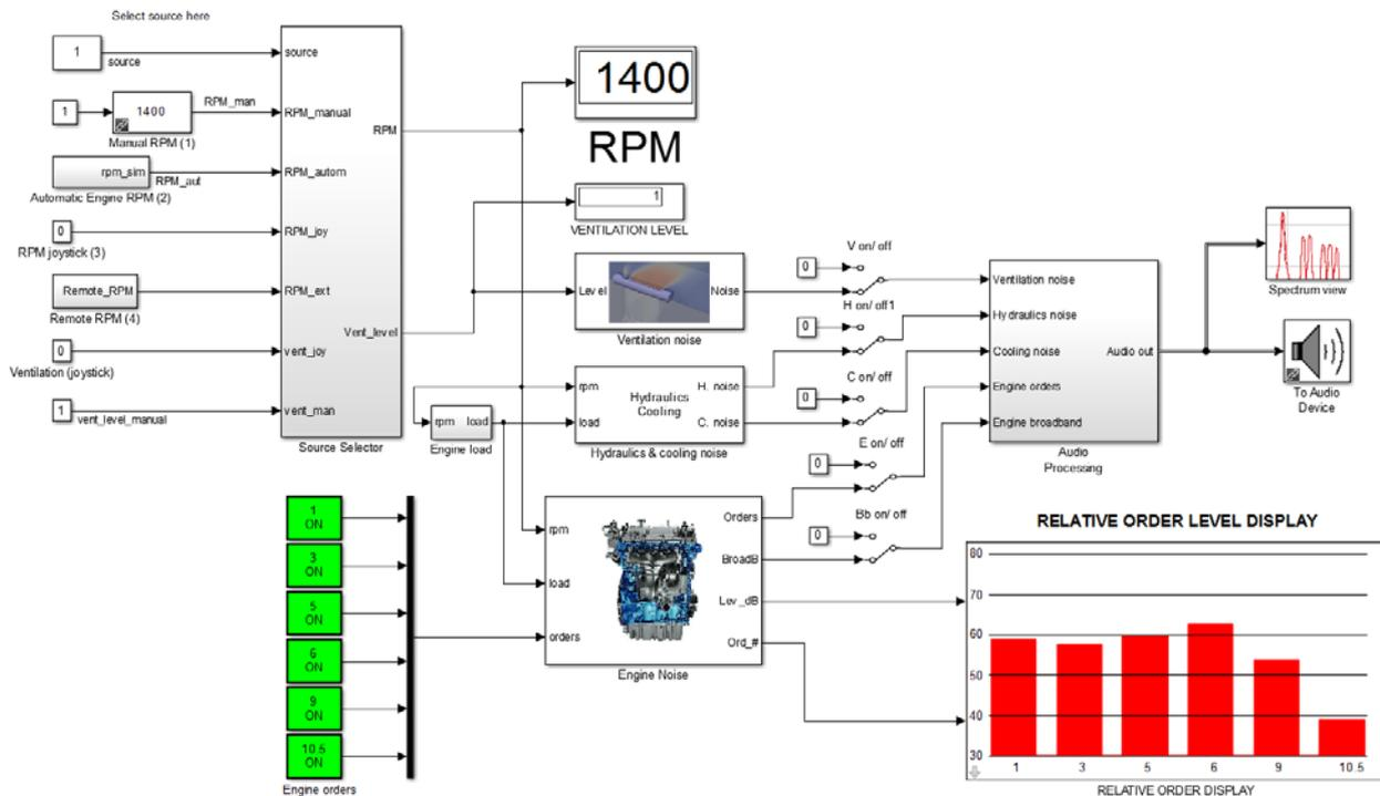
Figure 7: AMP-based simulation model realization for LHD cabin noise.
