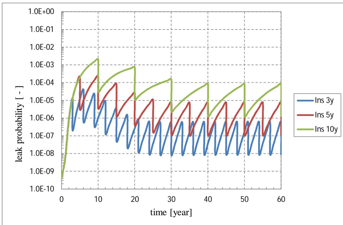
Figure 9. Leak probabilities with different inspection intervals for Medium pipe using IZPF POD curve.
