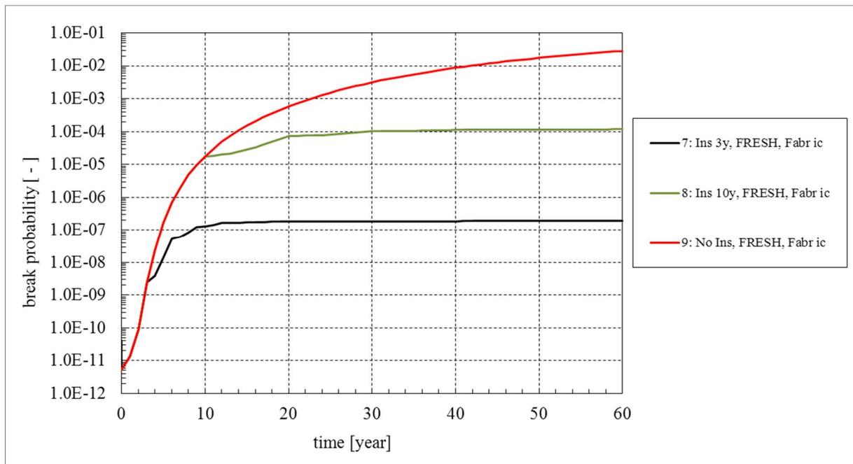
Figure 5. Break probability results for FRESH weld cross-section with FRESH WRSs from the third phase of the study [3].
