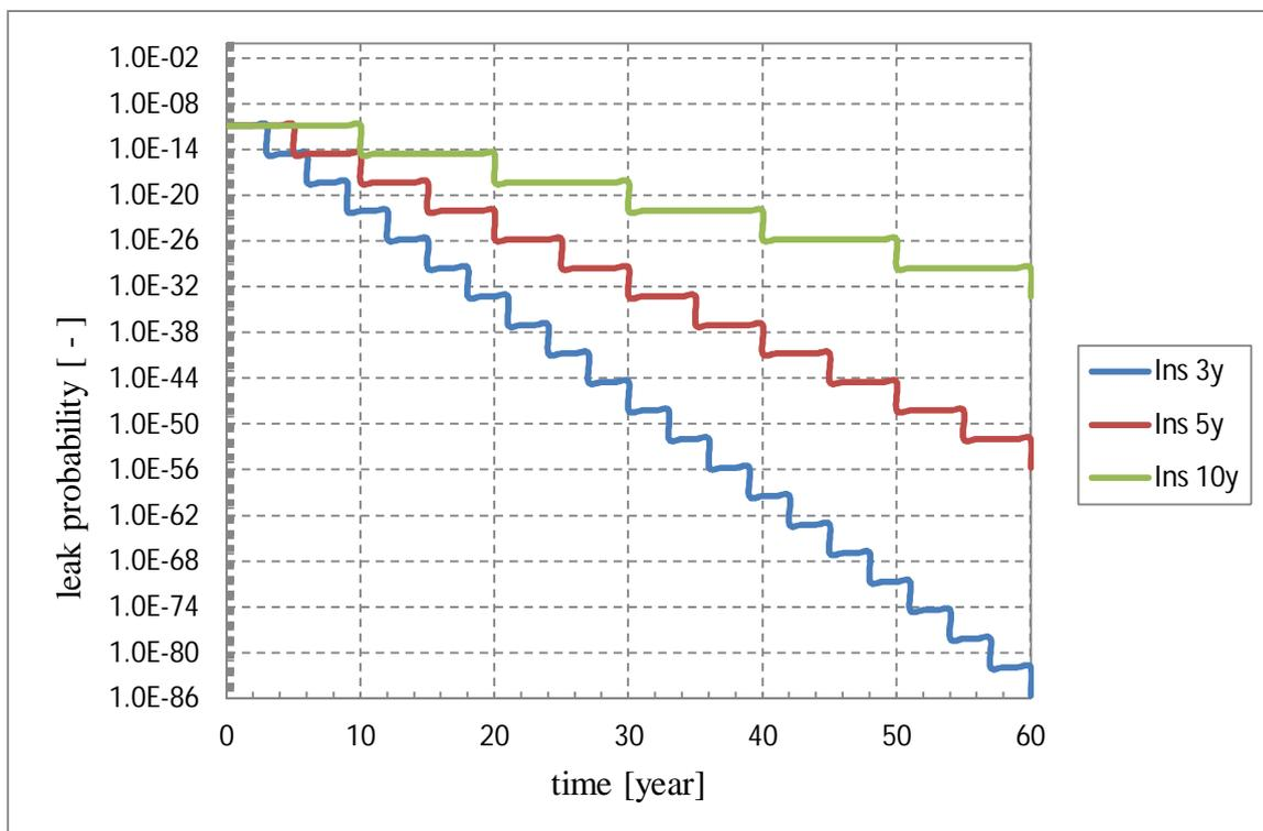
Figure 11. Leak probabilities with different inspection intervals for Large pipe using IZPF POD curve.
