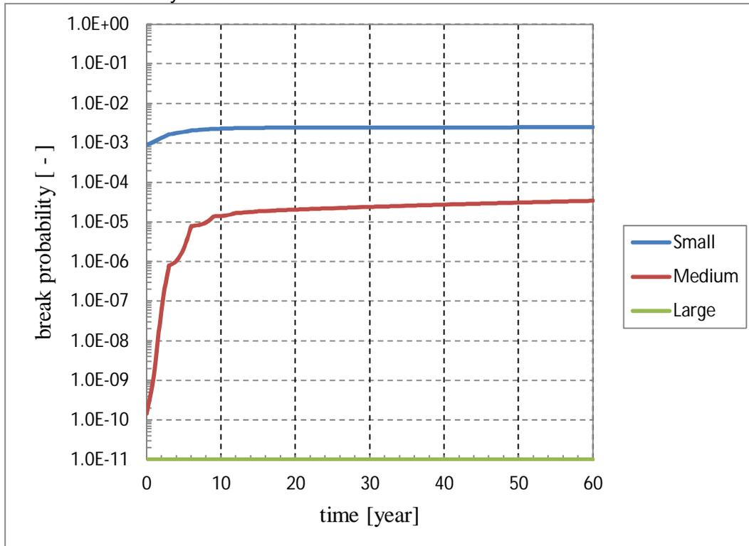
Figure 13. Break probabilities for different pipe sizes with IZPF POD curve and inspection interval of three years.
