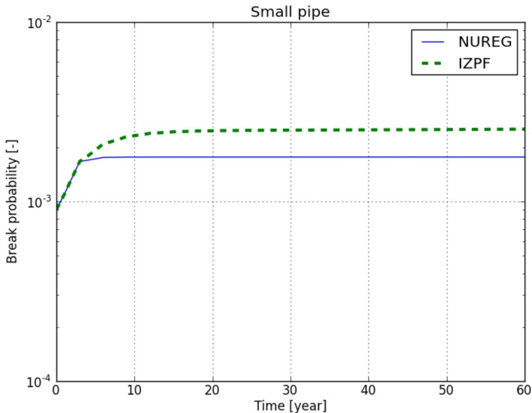
Figure 12. Break probabilities for Small pipe with different POD curves and inspection interval of three years.
