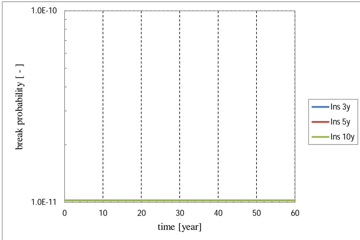
Figure 10. Break probabilities with different inspection intervals for Large pipe using IZPF POD curve.
