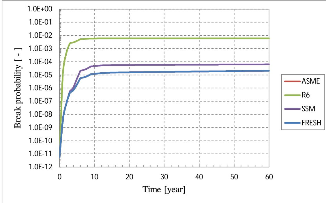
Figure 4. Break probability results for FRESH weld cross-section with different WRSs.
