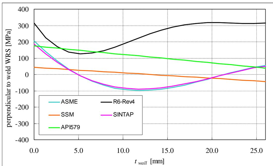
Figure 1: As-welded state WRS distributions through weld centre line and perpendicular to weld for Large pipe.
