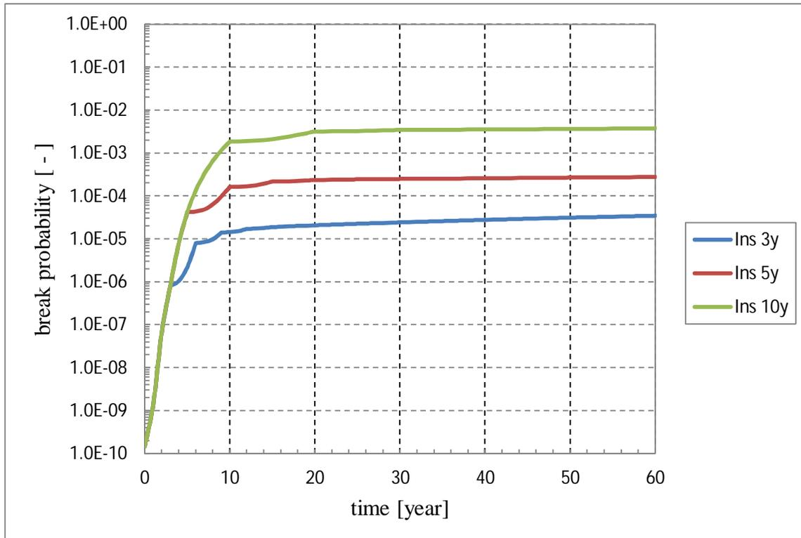
Figure 8. Break probabilities with different inspection intervals for Medium pipe using IZPF POD curve.
