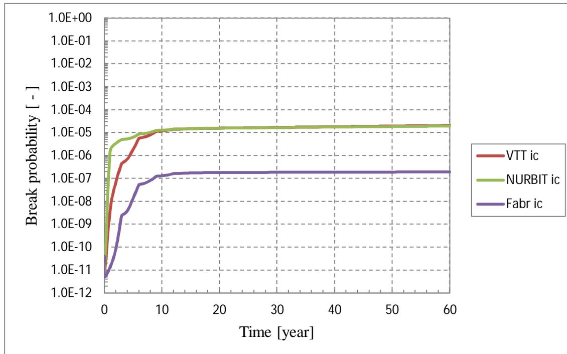
Figure 3. Break probability results for FRESH pipe component weld with different initial crack assumptions.
