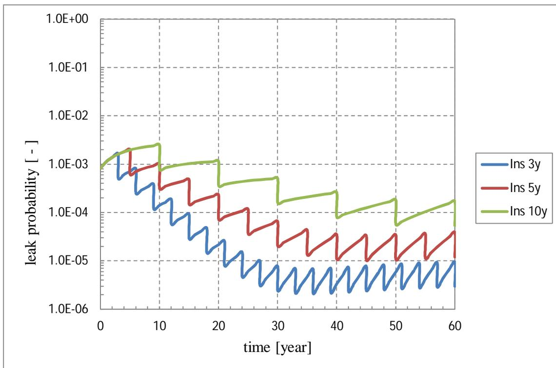
Figure 7. Leak probabilities with different inspection intervals for Small pipe using IZPF POD curve.
