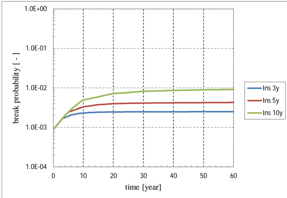
Figure 6. Break probabilities with different inspection intervals for Small pipe using IZPF POD curve.
