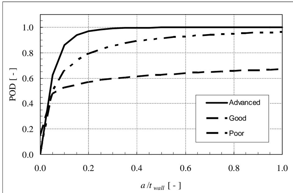
Figure 2: Distributions of POD function values concerning intergranular SCC for ferritic steel piping, according to NUREG/CR-3869 [20].
