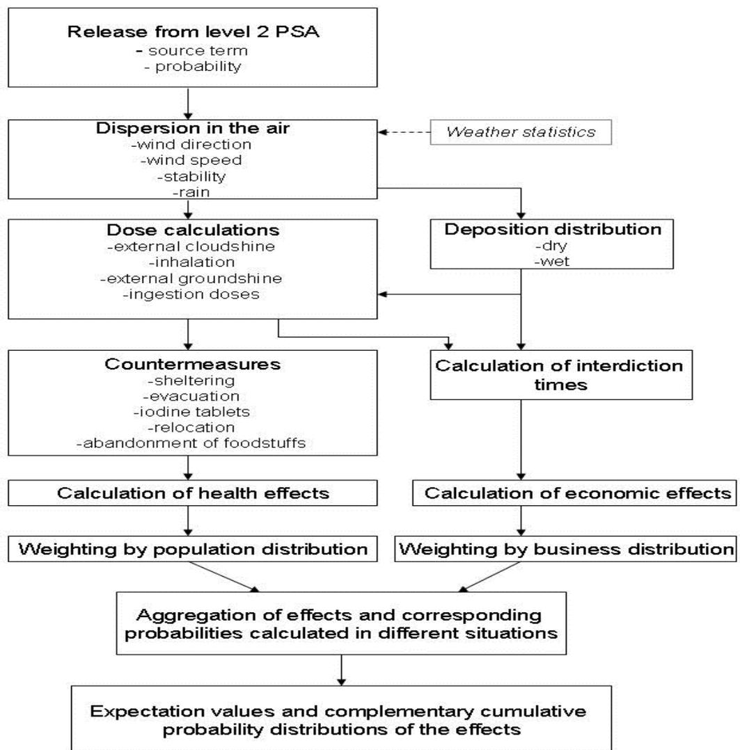
Figure 1. The flow chart of the ARANO computer code
