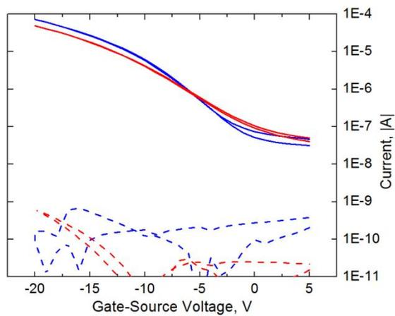
**Fig. 4.** A comparison of the transfer characteristics of spin coated (red) and printed (blue) transistors. Absolute drain current is shown with a solid line and the gate leakage current with a dashed line. Transistor channel length was 15  $\mu\text{m}$  and width 6870  $\mu\text{m}$ . The drain-source voltage was -20 V.
