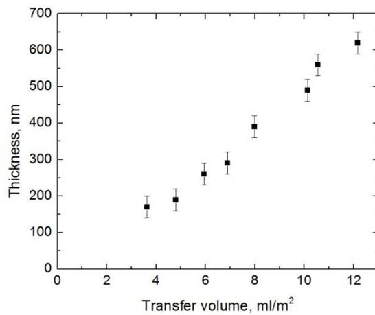
**Fig. 2. Gravure printed *Lisicon D320* dielectric film thickness for 8 different gravure plate transfer volumes.**
