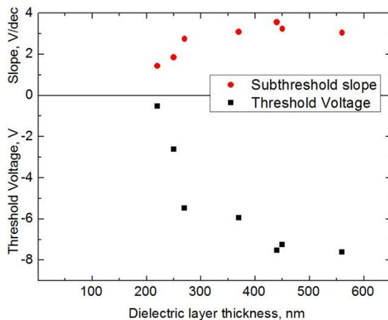
**Fig. 7. Printed transistor *subthreshold slope* (red) and *threshold voltage* (black) plotted versus the printed dielectric thickness.**
