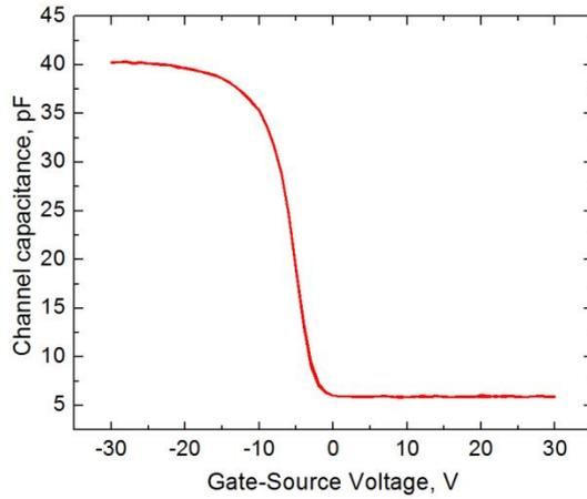
**Fig. 8. Overlapping forward and reverse sweeps of *capacitance-voltage* measurement at  $-20\text{ V}_{\text{DS}}$  show no indication of hysteresis or *threshold voltage shift*.**
