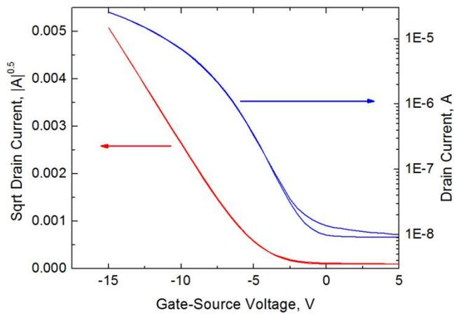
**Fig. 6. Printed transistor *transfer* ( $I_D$  vs.  $V_{GS}$ ) characteristics at -15  $V_{DS}$ . Transistor channel length was 15  $\mu\text{m}$  and width 6870  $\mu\text{m}$ .**
