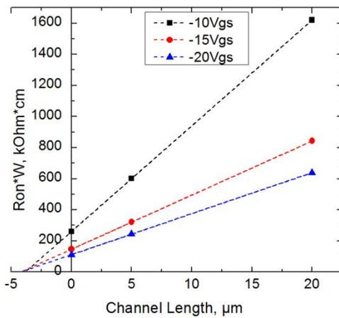
**Fig. 9. The plot shows an example of *channel* and *contact resistances* of a transistor at gate-source voltages  $V_{\text{GS}} = -10\text{ V}$ ,  $V_{\text{GS}} = -15\text{ V}$  and  $V_{\text{GS}} = -20\text{ V}$ . Drain-source voltage was  $-1\text{ V}$ .**
