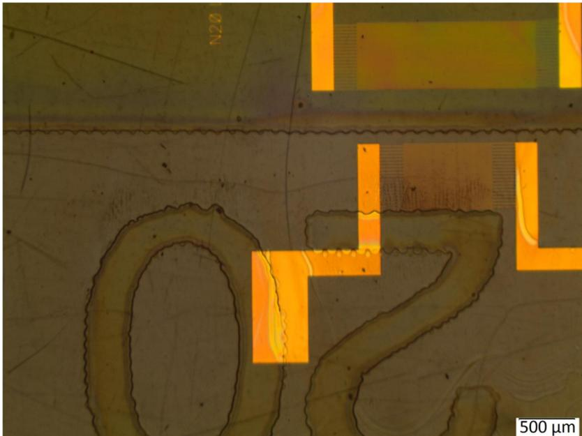
**Fig. 3.** Detail of a patterned feature printed with dielectric ink. Edge quality is following the gravure cell sizes. Printing line density was 120 lines/cm.
