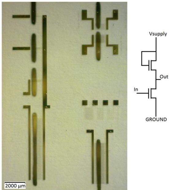
**Fig. 1. Photograph of transistors and inverter circuits and the inverter schematics.**
