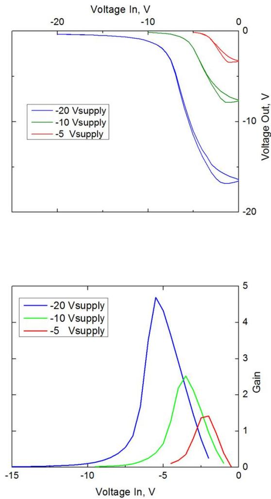
**Fig. 10.** The inverter worked at low voltages, shown by a) the *output swing* and b) corresponding *voltage gain* values at  $V_{\text{supply}} = -20\text{ V}$ ,  $V_{\text{supply}} = -10\text{ V}$  and  $V_{\text{supply}} = -5\text{ V}$ .
