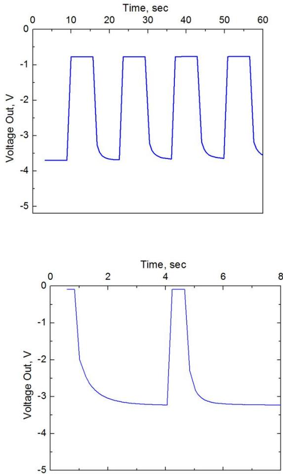
**Fig. 11.** Inverter dynamic characteristics are presented by the response to a 0 to -5 V *square wave* input signal. In a) the inverter had a *load:drive* size ratio of 1:10 and in b) 1:30. The long *On to Off* transition (closing) of the drive transistor is shown clearly. In b) the step time scale is different in order to show the full tail of the transition.
