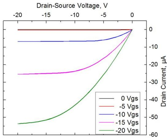
**Fig. 5. Printed transistor *output* characteristics. Transistor channel length was 15  $\mu\text{m}$  and width 6870  $\mu\text{m}$ .**
