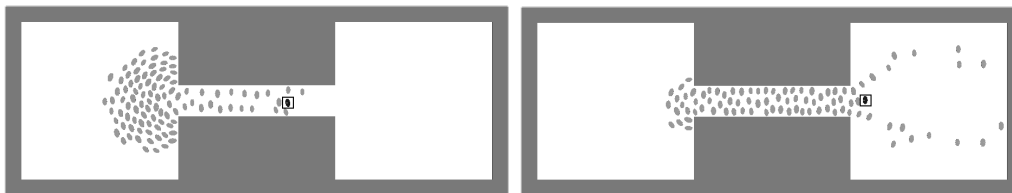
Figure 8: Snapshots of a simulation without the counterflow model. The single agent is black and highlighted with a square. The agents are unable to avoid collisions and the single agent gets pushed out of the corridor in an unrealistic manner.
