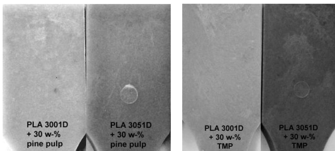
**Fig. 3** Colour differences of pine pulp and TMP composites depending on the PLA grade matrix
