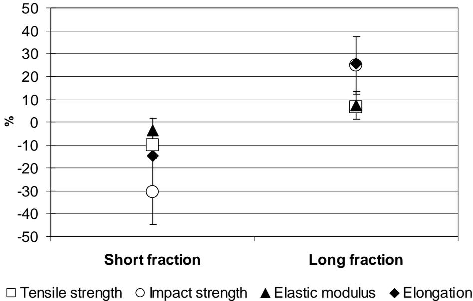
**Fig. 5 Effect of fractionation of TMP fibres on the mechanical properties of PLA composites containing 30 w-% fibres. The results are normalised with respect to composites containing TMP reference fibres (no fractioning).**
