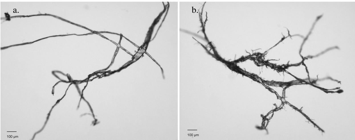
**Fig. 2** Light microscope images from dry pine pulp fibres at 50x magnification: a. unrefined fibres, b. 200 kWh-1 refined fibres
