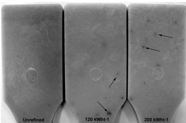
**Fig. 8 Macro-scale fibre dispersion of unrefined and refined pine pulp fibres in a PLA matrix with a fibre content of 30 w-%**
