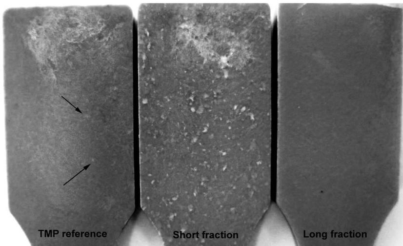
**Fig. 6 Macro-scale fibre dispersion of unfractionated and fractionated (short and long fractions) TMP fibres in a PLA matrix with a fibre content of 30 w-%**
