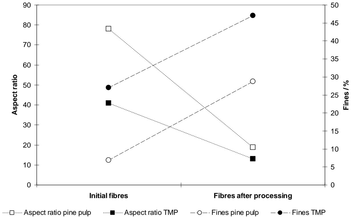
**Fig. 4 Effect of processing (compounding and injection moulding) on the aspect ratios and fines contents of pine pulp and TMP fibres. To measure the fibres after processing, the PLA 3051D matrix was dissolved from the injection-moulded specimen and the remaining fibres were analysed.**
