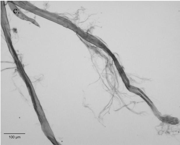
**Fig. 1** Light microscope images from wet and stained pine pulp fibres at 100x magnification: a. unrefined fibres, b. 120 kWh-1 refined fibres, c. 200 kWh-1 refined fibres
