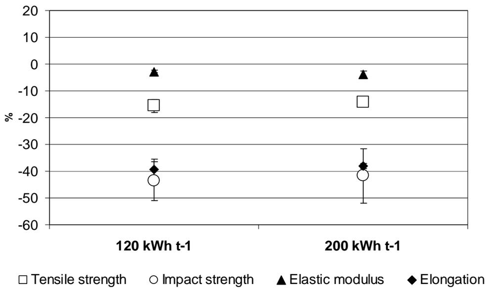
**Fig. 7 Effect of refining pine pulp fibres on the mechanical properties of PLA composites containing 30 w-% fibres. The results are normalised with respect to composite containing pine pulp reference fibres (no refining).**
