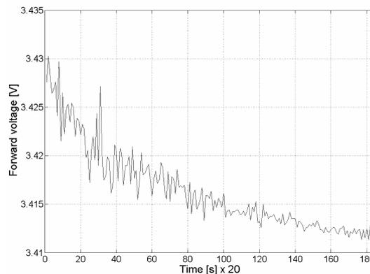
Figure 11: Forward Voltage of Blue LED on 1 mm Thick Alumina Substrate.
