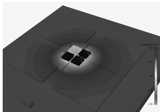
**Figure 4: Simulated Surface Temperatures of Prototype Module with 1-mm Thick Substrate.**
