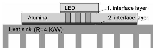
**Figure 2: Interface Layers of Simulated Structure.**
