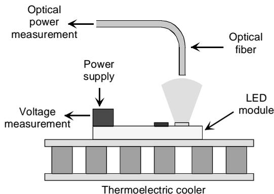
Figure 9: Measurement Setup for LED Modules.
