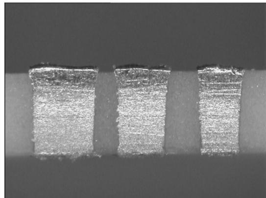
**Figure 7: Sintered and Diced Via Plugs with Diameter of 0.4 mm, 0.3 mm and 0.25 mm. Substrate thickness is 0.5 mm.**
