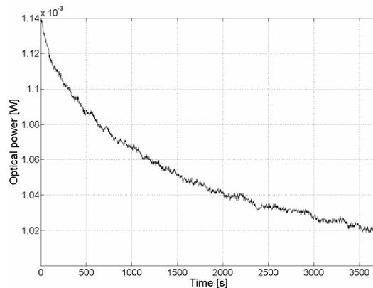
Figure 10: Optical Power of Blue LED on 1 mm Thick Alumina Substrate.
