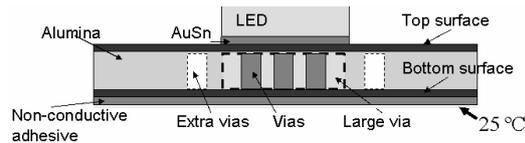
**Figure 3: Simulated Structure with Variations of Thermal Vias and Heat Distribution Layers.**
