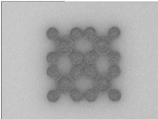
**Figure 5: Thermal Via Structure for 2×2 LED Array on 0.5-mm Thick Alumina Substrate. Via diameters are 0.4 mm and 0.25 mm.**
