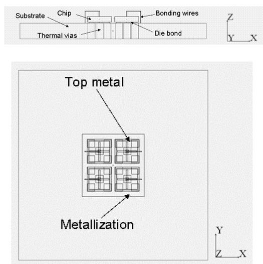
**Figure 1: Thermal Model of LED Module.**
