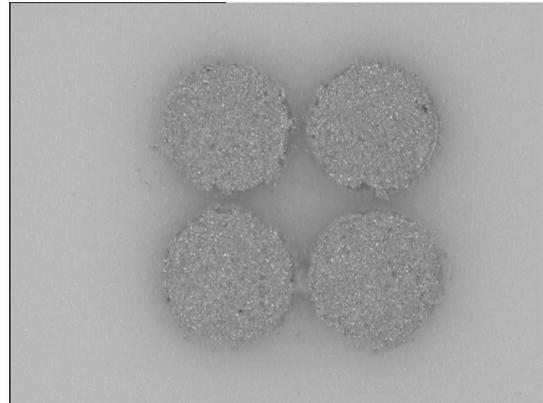
**Figure 6: Thermal Via Structure for 2×2 LED Array on 0.63 mm Thick Alumina Substrate. Via Diameter is 0.9 mm.**
