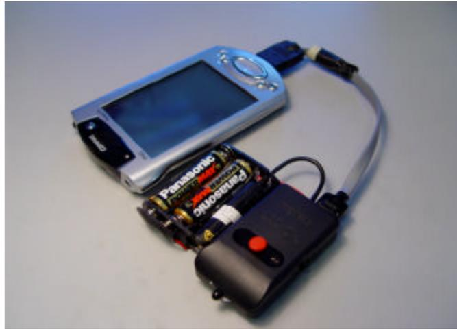
**Fig. 2.** The physical browser components: iPAQ (left), central SoapBox (right) and a laser beam unit (middle). The SoapBox has a pointing button (shown in the middle of the SoapBox) to activate the laser unit and the IR-transmitter (visible in front of the SoapBox)
