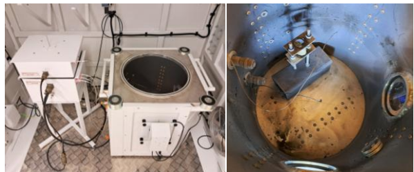
Standard calorimeter (left) and Cylindrical cell stand inside the EV+ calorimeter.
