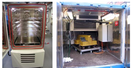
Thermal chamber (left) and interior of the climate container (right)
