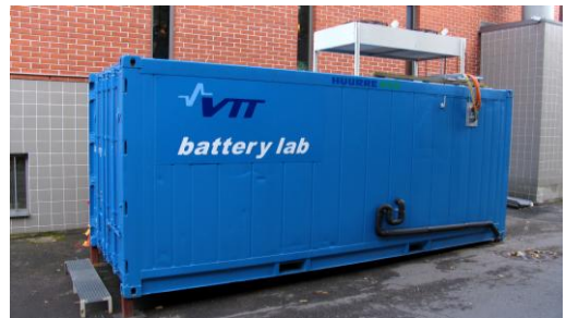
Climate container for battery pack testing
