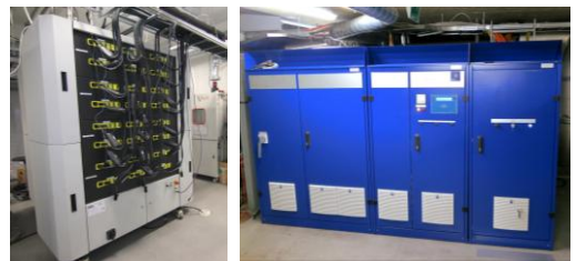
PEC cell tester (left) and AVL battery pack cyclor / emulator (right)
