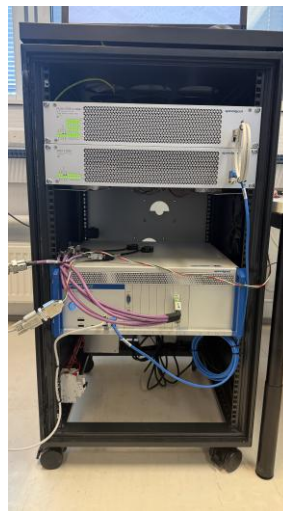
Speedgoat P3 Machine with BCE and FIU/TSE emulator (front end and back end)
