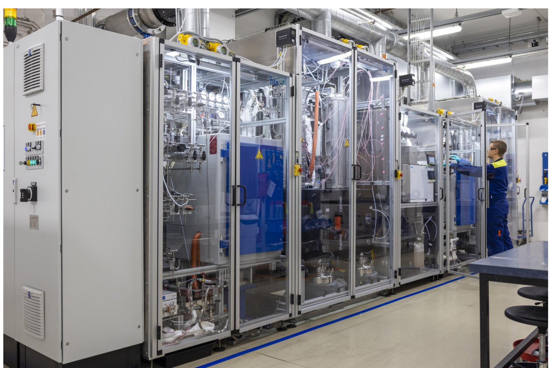
High-throughput test unit with 4 parallel fixed-bed reactors.
