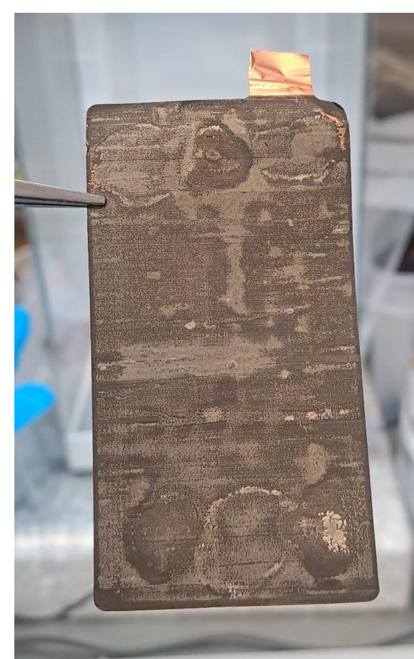
Lithium plating on graphite electrode
