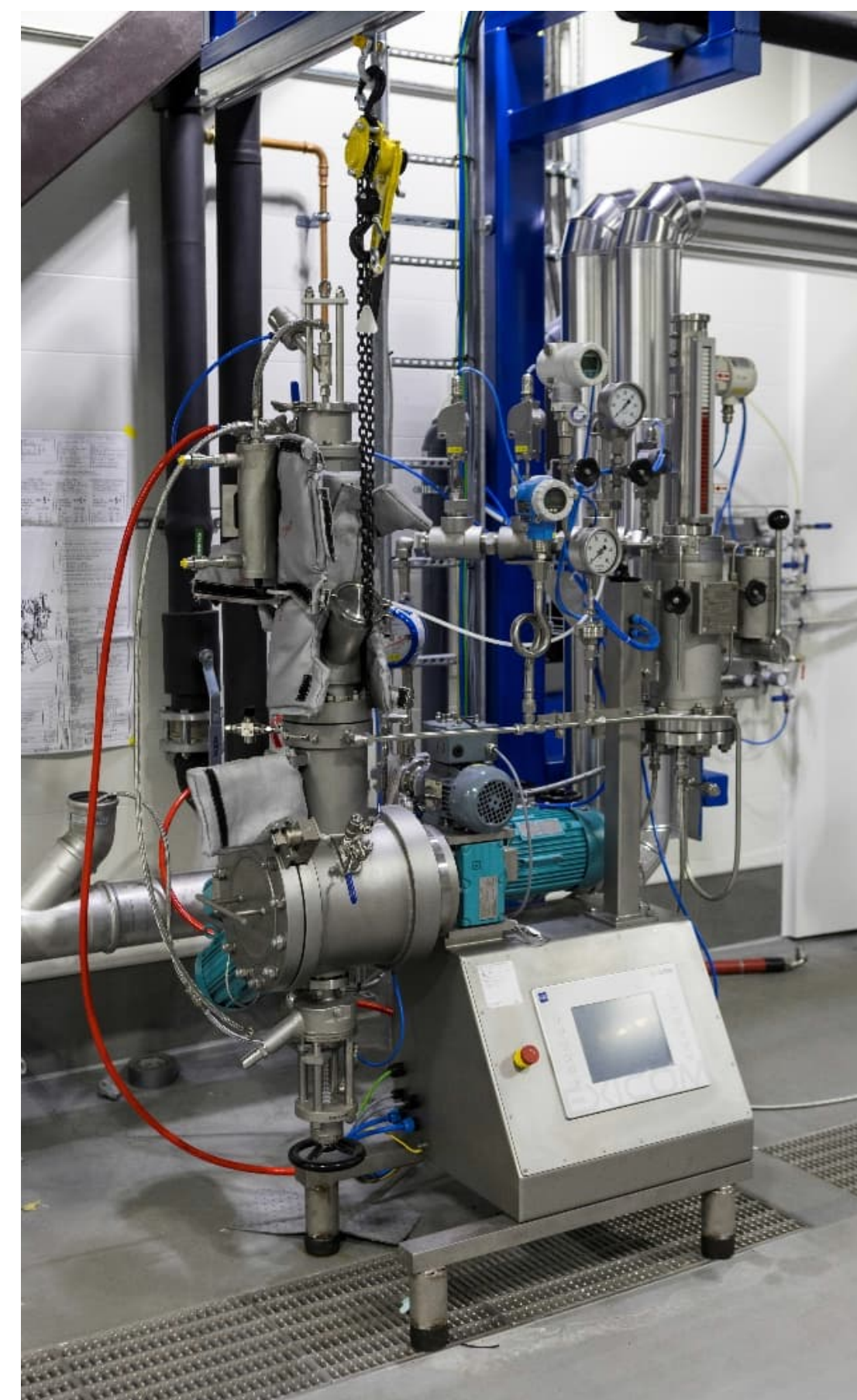
Fully EX proof multimaterial pilot platform with reactors and separation devices to allow flexible process demonstration and scale-up
