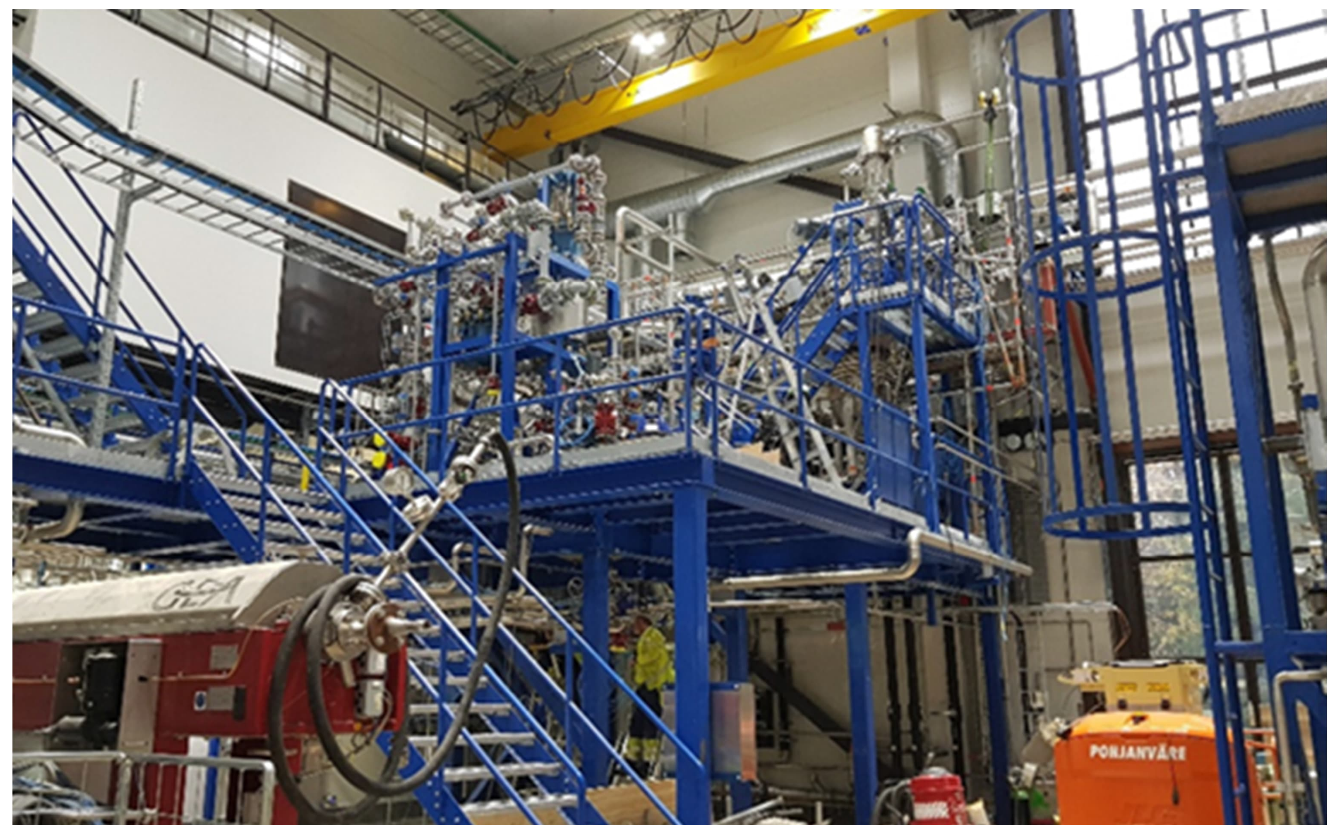
Fully EX proof multimaterial pilot platform with reactors and separation devices to allow flexible process demonstration and scale-up
