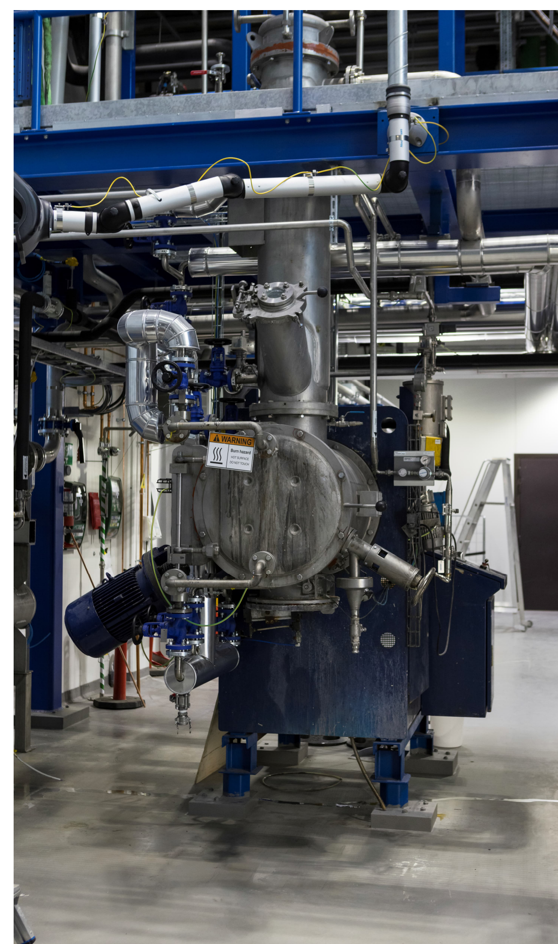
Multistage processing in batch, high speed reactors allowing step wise scale up with fixed parameters from 5 L to 600 L scale. Typically used for
