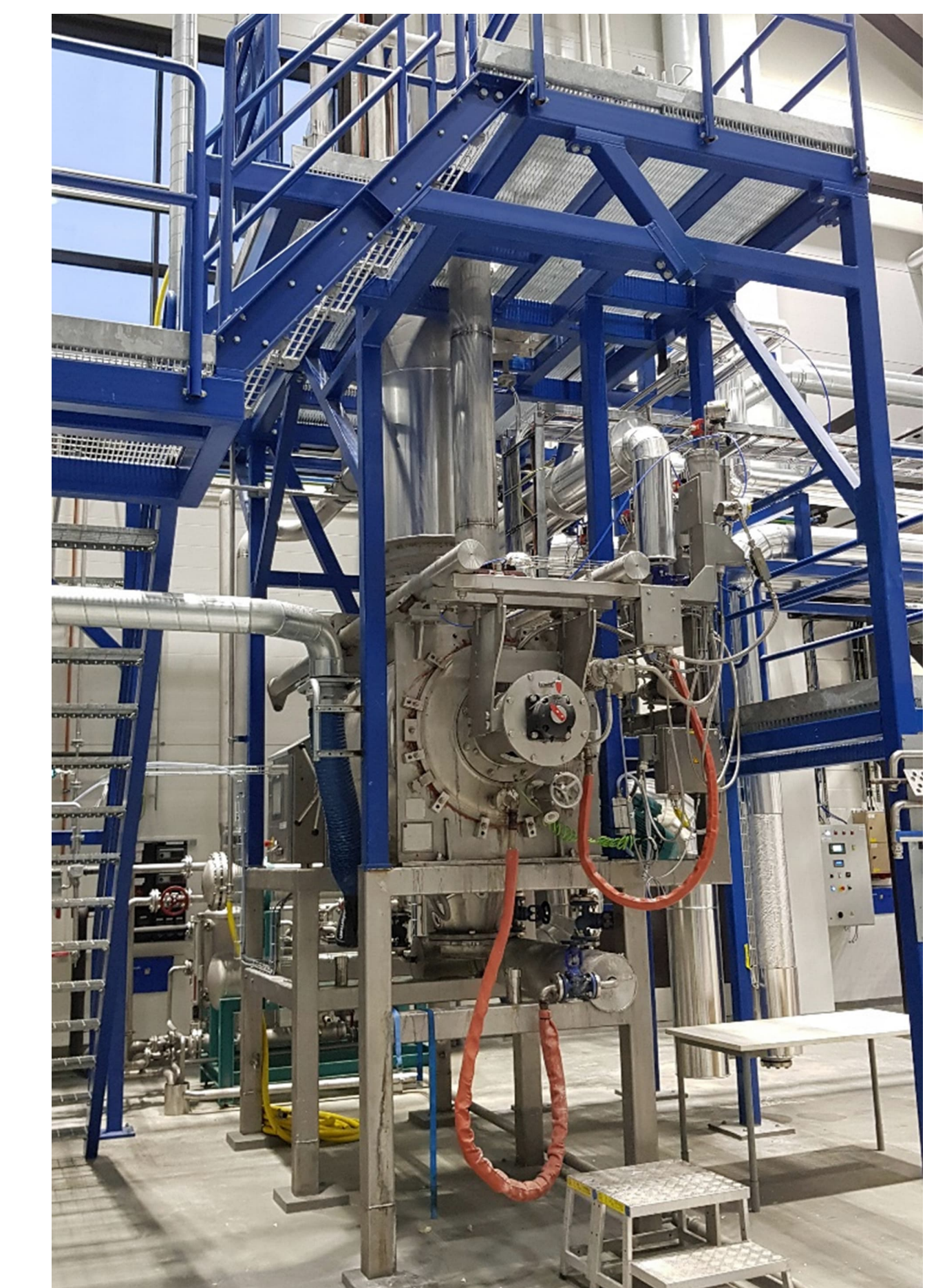
Multistage processing in batch, high speed reactors allowing step wise scale up with fixed parameters from 5 L to 600 L scale. Typically used for
