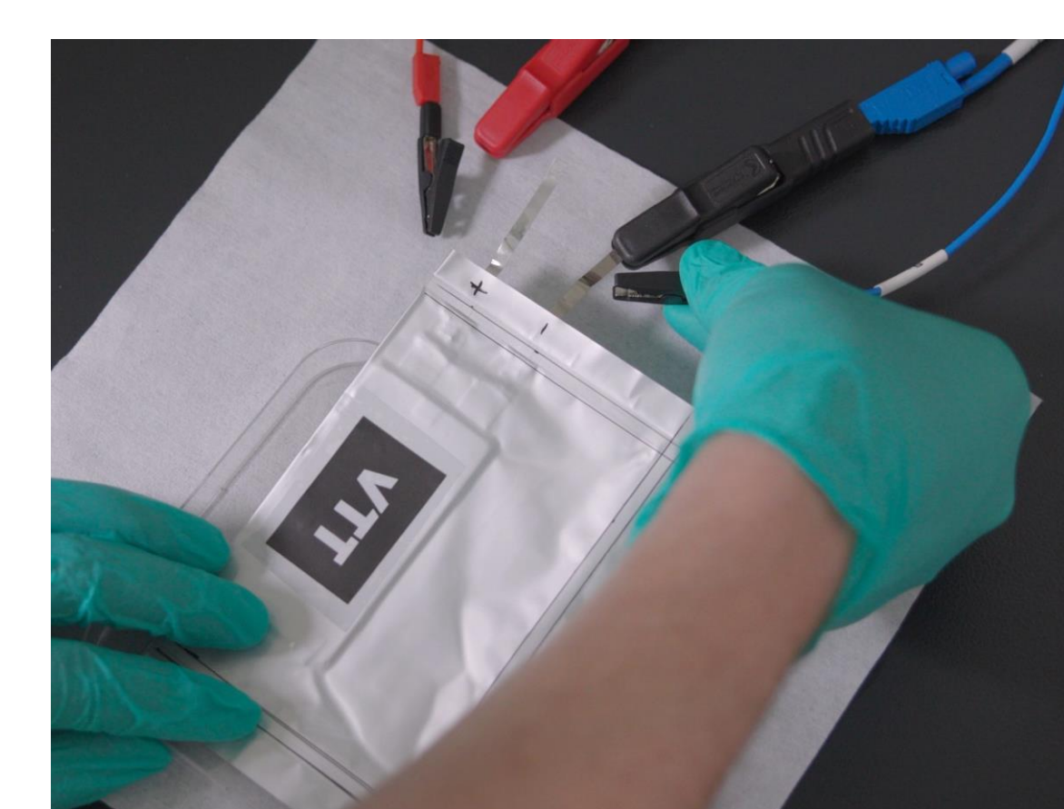
Pouch cell layers and a ready cell
