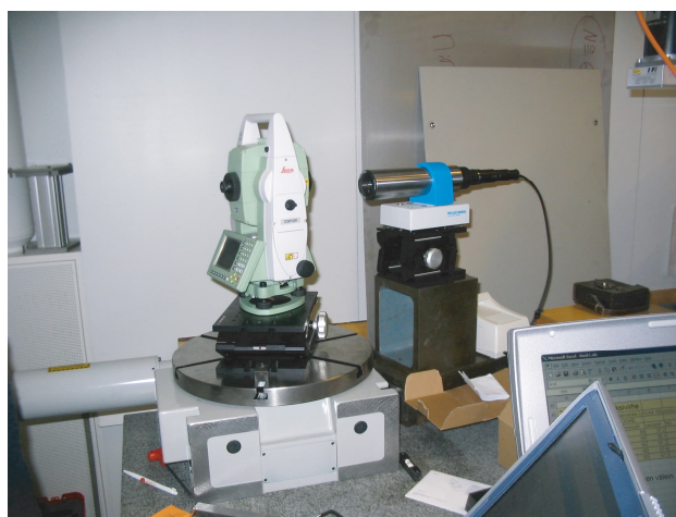
Figure 2. Calibration of the horizontal plane of a tachymeter in an Eimeldingen rotary table with a collimation tube as a target point.
