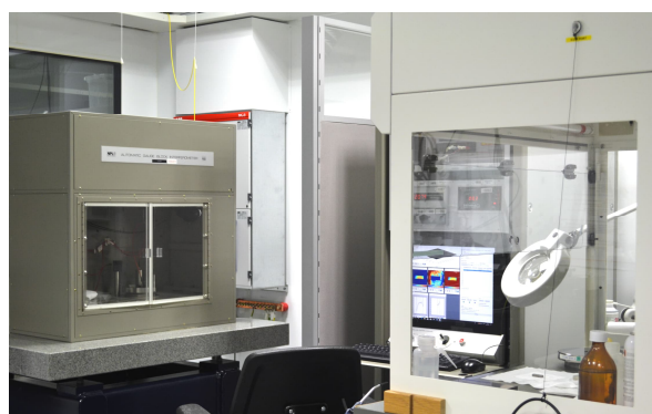
Figure 1. VTT MIKES PSIGB gauge block interferometer and wringing station.
