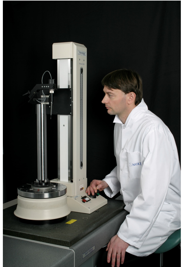
Figure 2. Measurement instrument Talyrond 262 for roundness and cylindricity.
