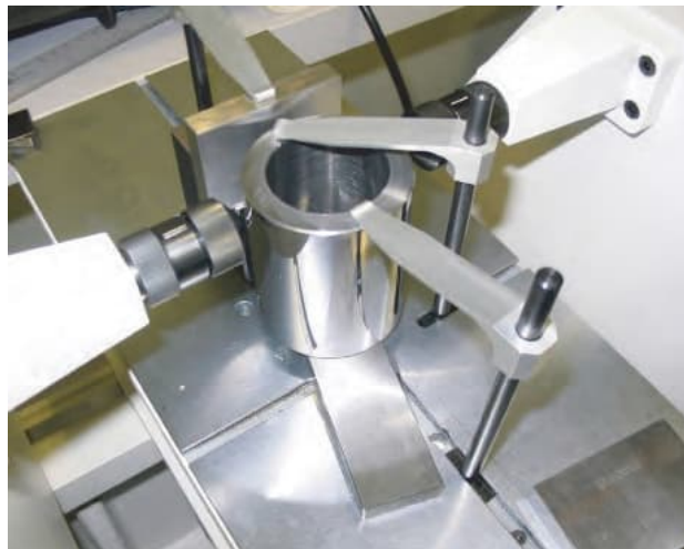
Figure 2. Mounting side by side the artefact under calibration and the reference in a comparison measurement.
