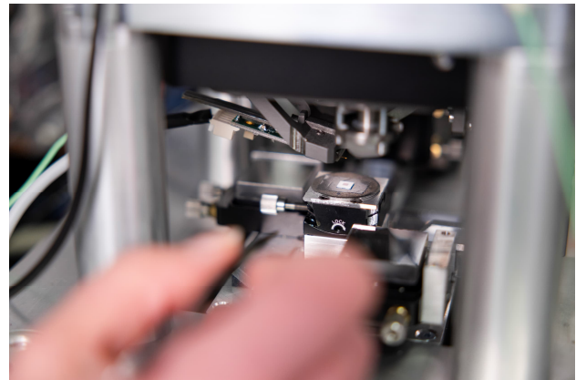
Figure 2. Interferometrically traceable MIKES metrological AFM.
