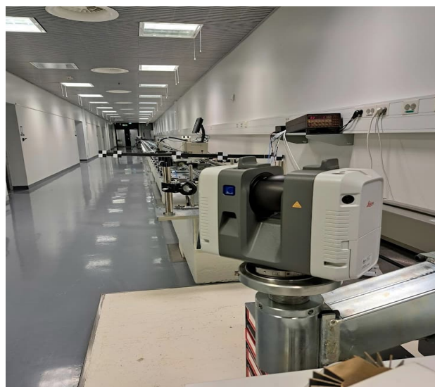
Figure 1. Calibration of a laser scanner with a 30-metre measuring rail.
