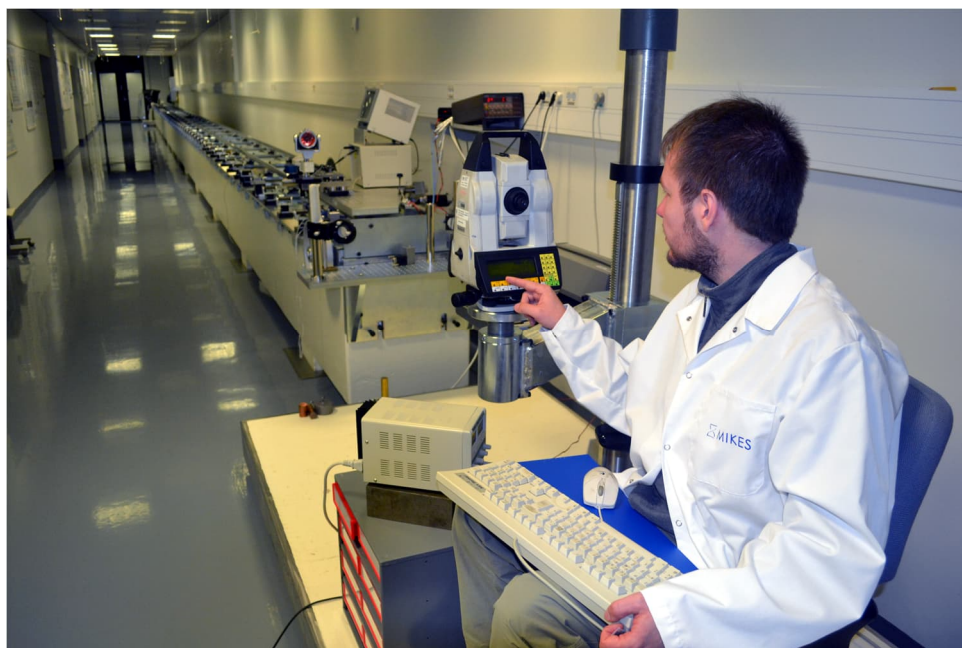
Figure 1. MIKES 30-m measuring rail.
