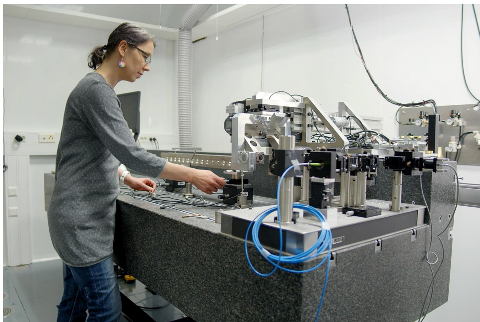
Figure 1. VTT MIKES interferometer for calibration of step gauges.
