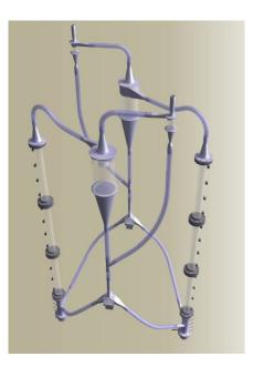
Figure 27. 3D rendered image of the equipment built for solid circulation and hydrodymanics testing at VTT (Tähtinen et al., 2012).
