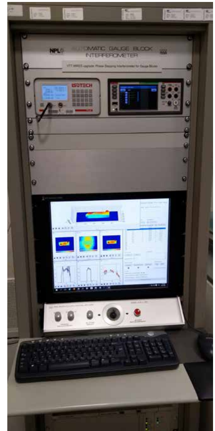
Figure 3. Upgraded electronics cabinet and GBI software.
