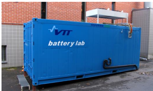
Climate container for battery pack testing
