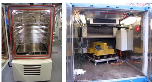
Thermal chamber (left) and interior of the climate container (right)
