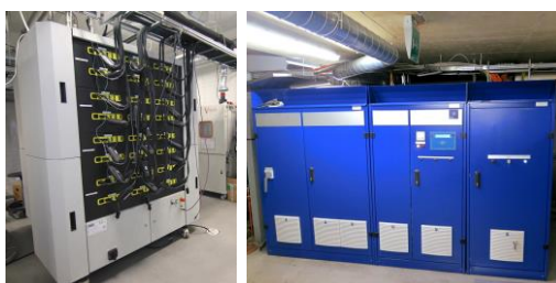
PEC cell tester (left) and AVL battery pack cyclor / emulator (right)
