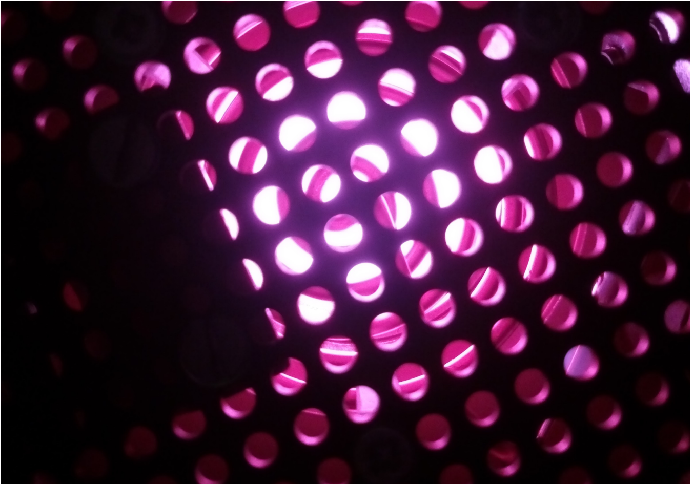
Hydrogen glow from H_2 dissociator, from one of VTT MIKES active hydrogen masers.
