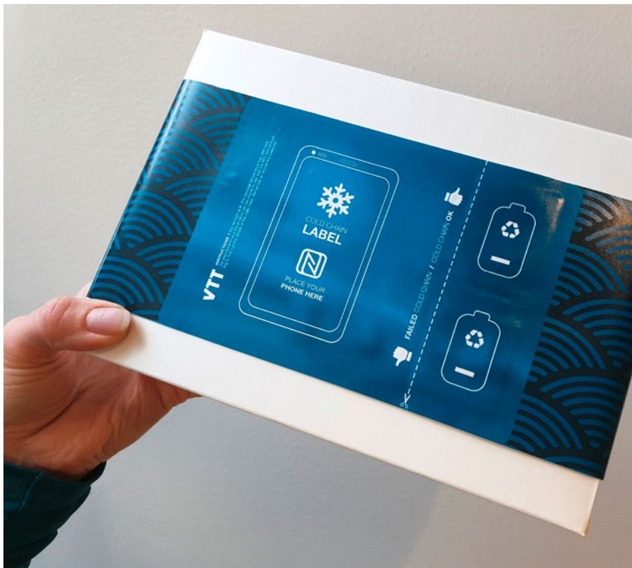
Figure 2: A smart data logger label demonstrator (T-tag9, developed by VTT)
