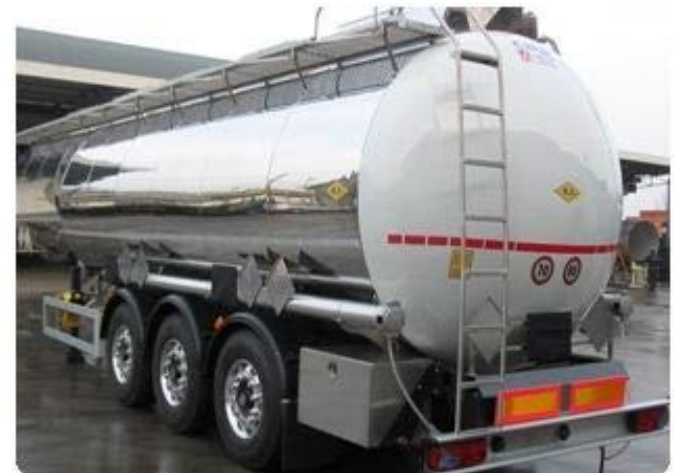
A bitumen road tanker using LDX 2101®
