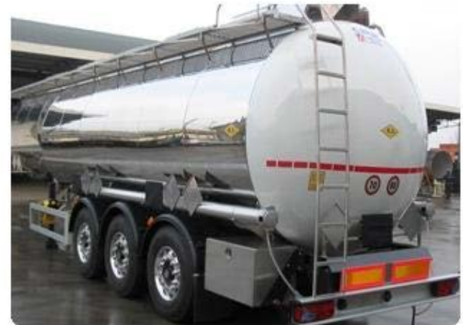
A bitumen road tanker using LDX 2101® Photo courtesy of manufactured by Officine Meccaniche B.S. S.r.l.
