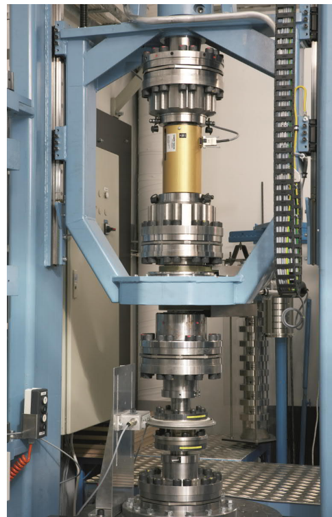
Figure 3. A 20-kNm torque standard based on a reference sensor.
