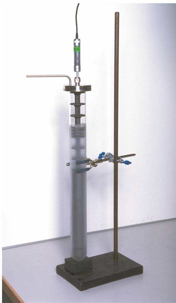
Figure 1. Pt25-sensor (SPRT) in a fixed-point cell.
