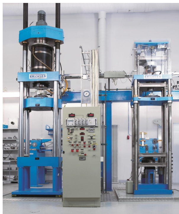
Figure 1. The 1-MN hydraulic amplification force standard machine and the 100-kN deadweight force standard machine. The total equipment height is eight meters, including the deadweights below floor level.
