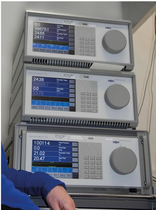
Figure 1. Calibration of chilled mirror hygrometers.
