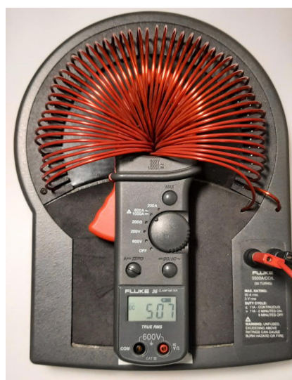
Figure 2. Clamp current meter in a 50-turn calibration coil measuring a large 500 A direct current.
