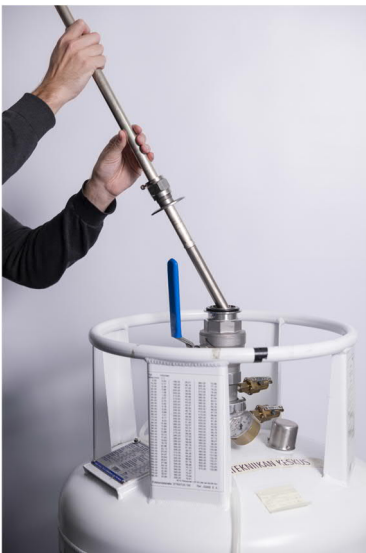
Figure 1. The traceability of direct current is based on a Josephson standard cooled in liquid helium.
