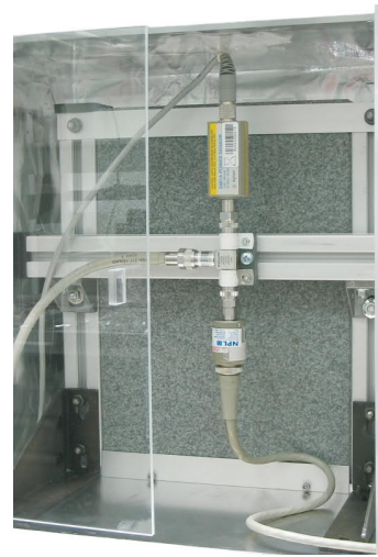
Figure 2. Measurement set-up for power sensors.
