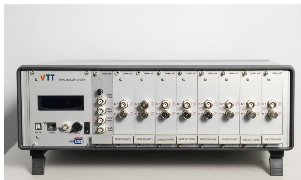
Figure 1. Six channel sampler for power calibrations. The sampler can be used also for calibration of power harmonics, and digital measuring instruments using IEC 61850-9-2 LE and IEC 61869-9 protocols.
